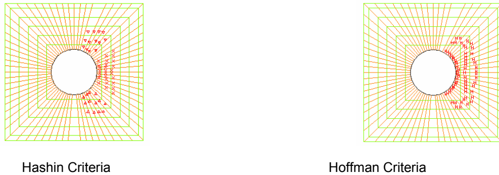
Figure 5.6 Illustration of Damage Propagation ( E/D=4 ; W/D=4 ; \Theta=0 )
