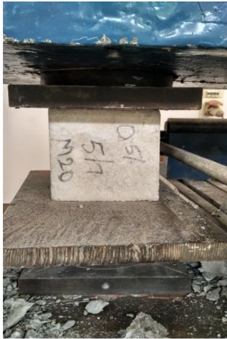
Figure 3. 4 Concrete cubes under compression testing machine
