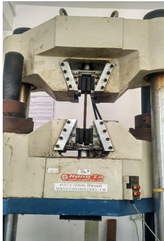
Figure 3. 3 Testing of steel reinforcement
