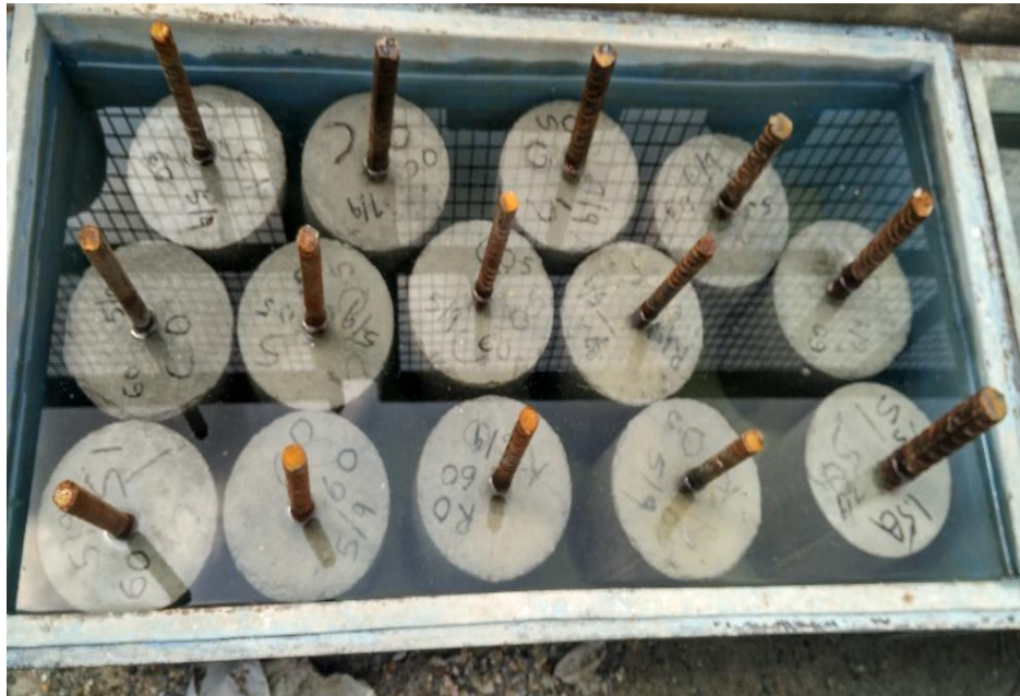
Figure 3. 8 Curing of pull-out specimens
