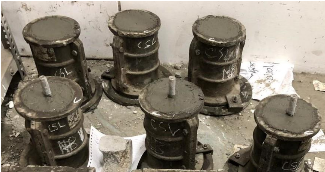
Fig. 3.14: Steel bars embedded in concrete samples at the time of casting
