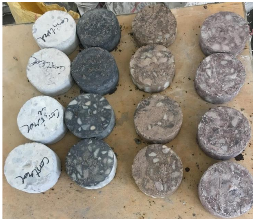
Fig. 3.18: Prepared samples for sorptivity test
