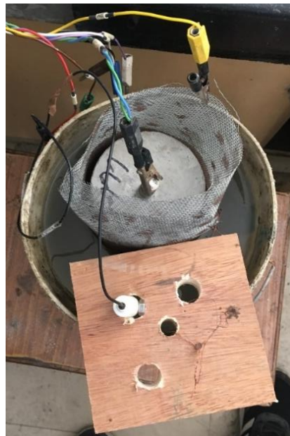
Fig. 3.25: Connections on steel embedded concrete samples for electrochemical tests
