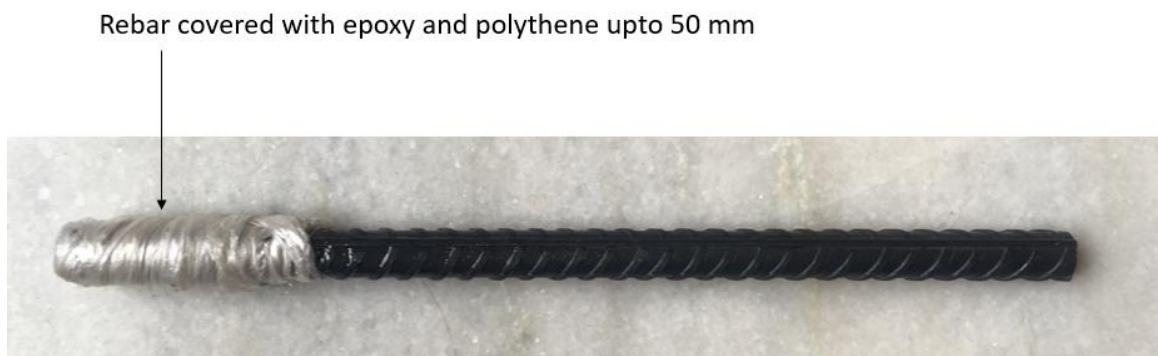
Fig. 3.12: Steel rebars used in concrete tests marked for application of epoxy
