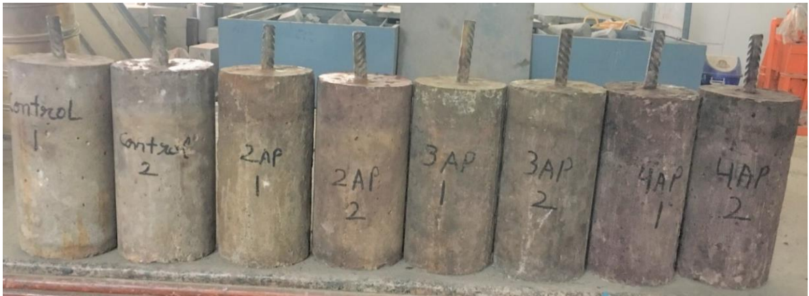
Fig. 3.17: Prepared steel embedded cylindrical concrete samples for electrochemical tests
