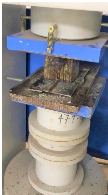
Fig. 3.21: Splitting of cubes for carbonation depth test
