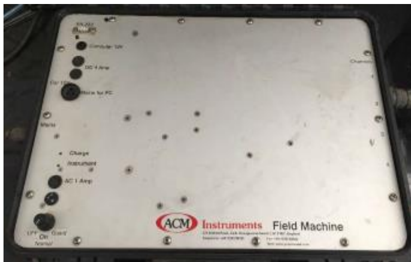
Fig. 3.7: ACM field Machine serial no. 1463 used for electrochemical tests
