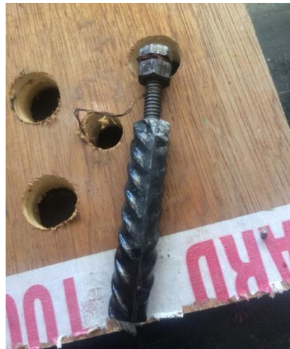
Fig. 3.6: Prepared steel sample attached with wooden lid
