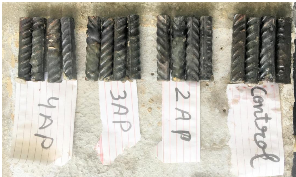
Fig. 3.11: Steel samples after LPR test in carbonated pore solution
