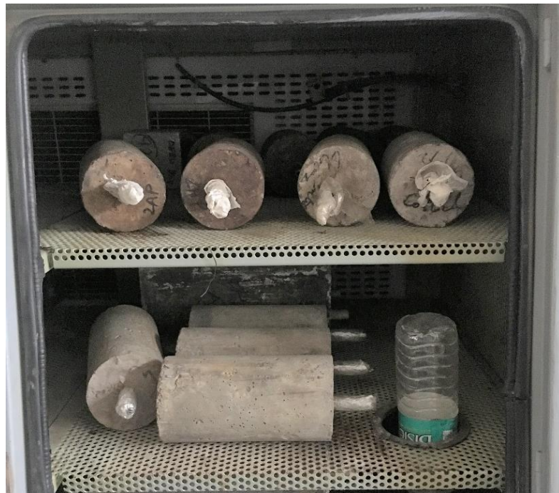
Fig. 3.19: Concrete samples subjected to accelerated carbonation inside carbonation chamber
