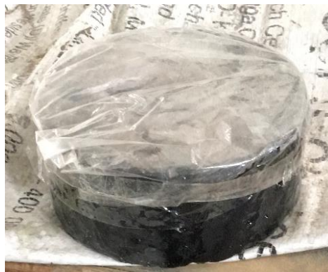
Fig. 3.15: Sample prepared for Sorptivity test covered with loose plastic sheet and epoxy
