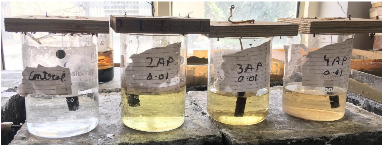
Fig. 3.4: Steel samples immersed in prepared solution after 24 hours
