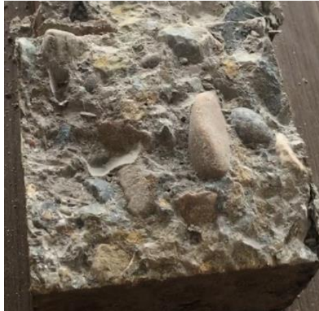
Fig. 3.22: Cube split from middle for carbonation depth
