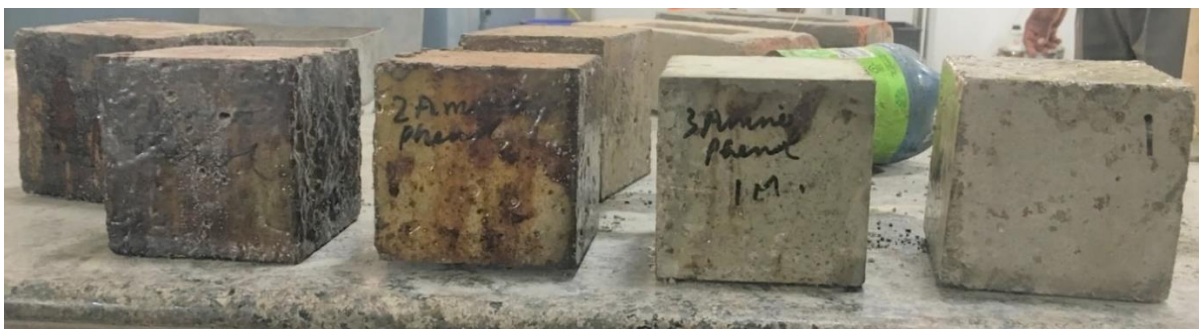
Fig. 3.16: Prepared cubical samples for carbonation depth test
