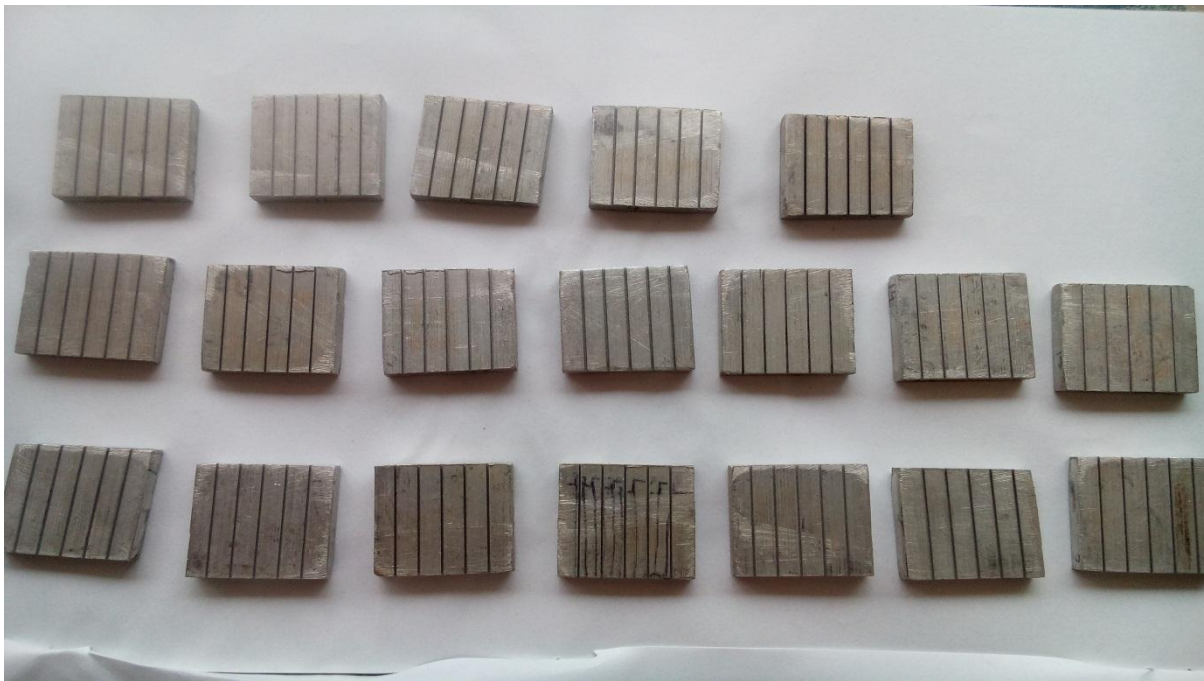
Fig 3.12 Shows 20 specimens on which micro channels are formed with different 20 parameter settings using Wire EDM.
