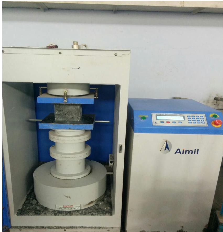
Fig. 4.1: Compressive strength test setup
