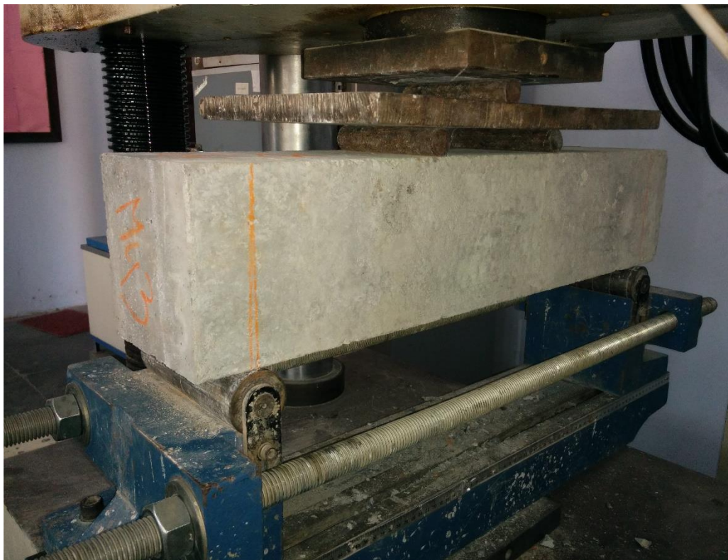
Fig. 4.8: Test setup for flexural strength
