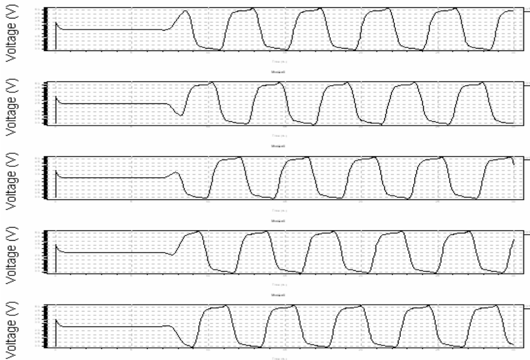
Figure 5.2 Waveform obtained after the transient analysis of ring oscillator.
