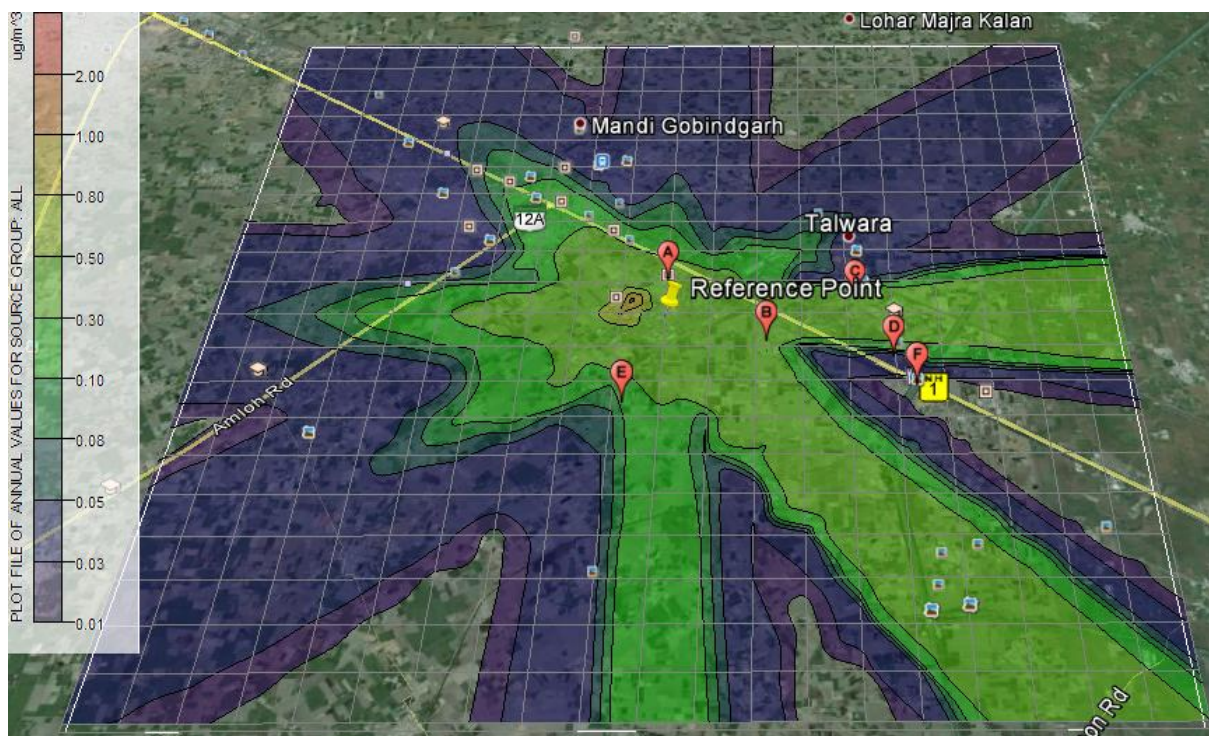
Figure 5.6: Isopleths showing dispersion of NO 2 for 24h averaging time
