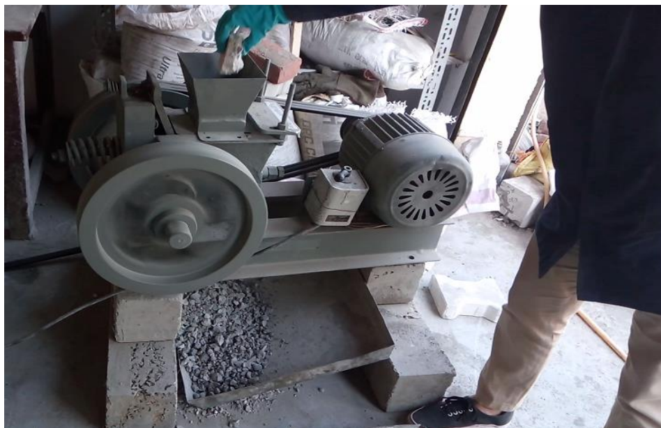
Figure 3.4: Using a jaw crusher to make recycled coarse aggregates
