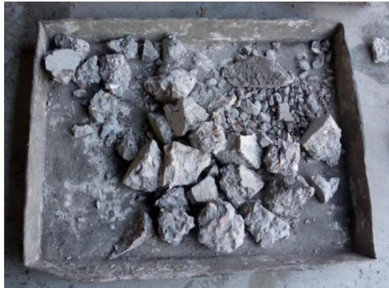
Figure 3.3: Waste concrete pieces used for making recycled coarse aggregates
