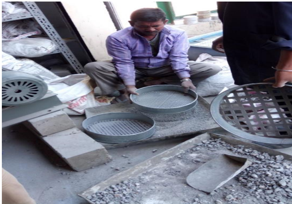
Figure 3.5: Sieving work after making recycled coarse aggregates with jaw crusher
