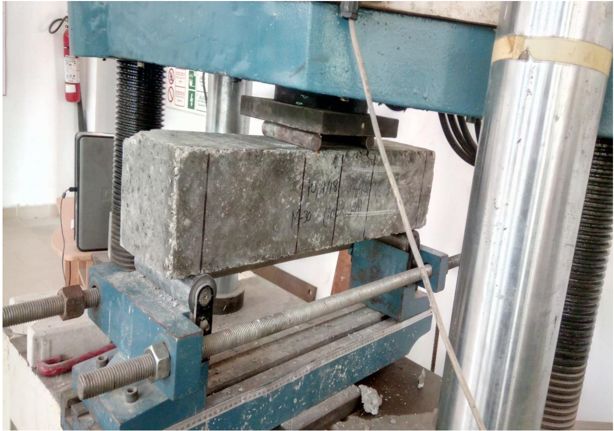
Figure 3.16: Testing of a beam for flexural strength on UTM
