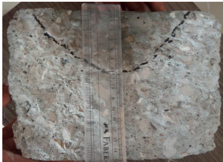
Figure 3.22: Measuring the water penetration depth with scale
