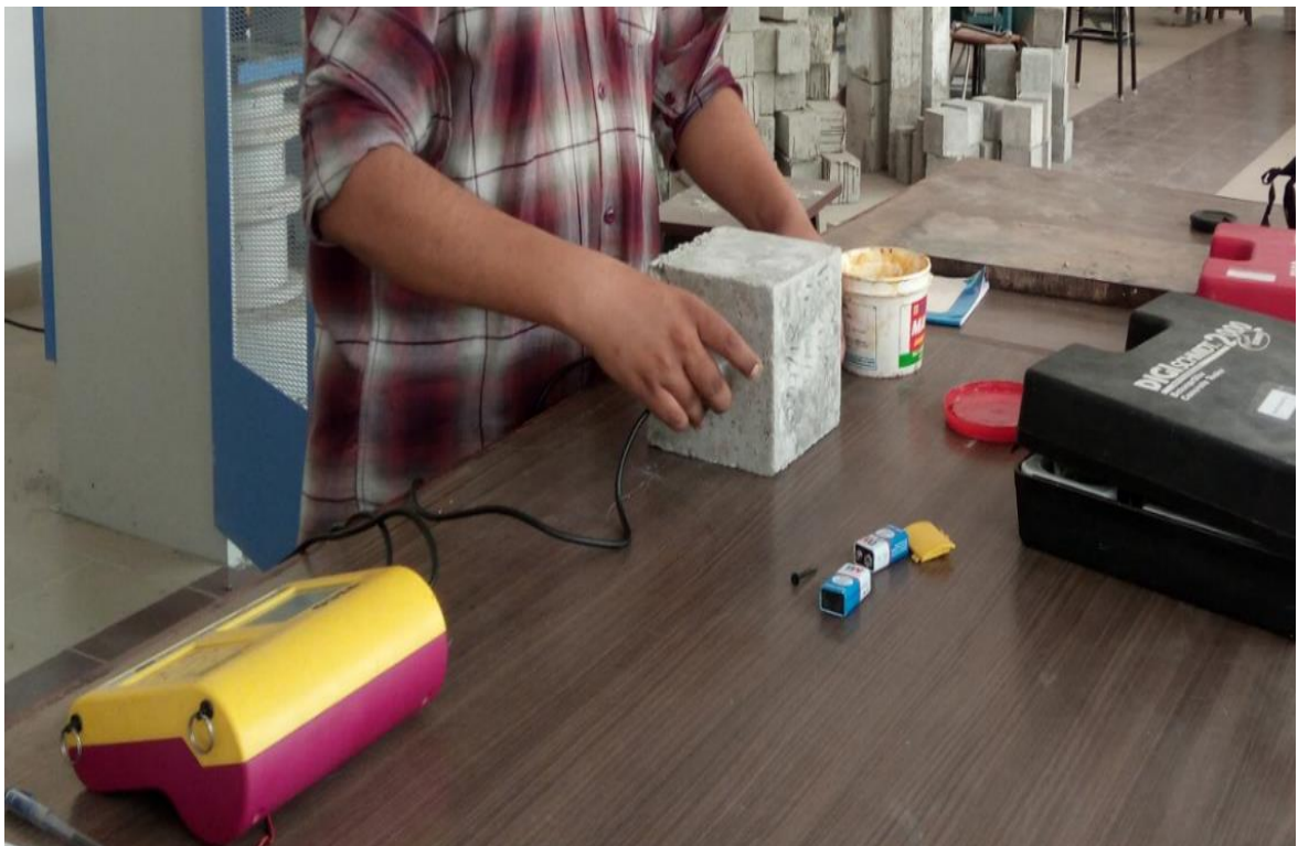
Figure 3.12: Testing set up for determining ultrasonic pulse velocity through concrete
