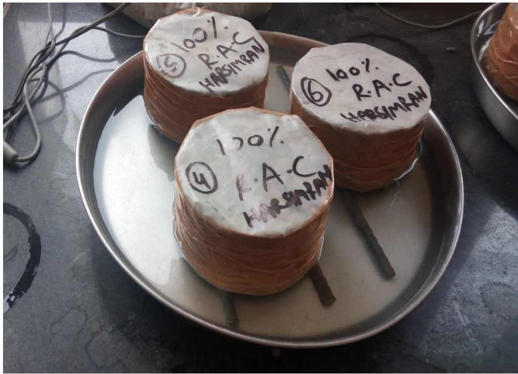
Figure 3.23: Testing setup for performing sorptivity of concrete specimens
