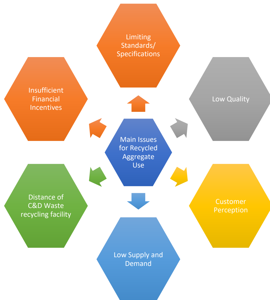
Figure 1.13: Problems associated with the recycled aggregate that prevent its wider use in construction, (Tam et al., 2018)
