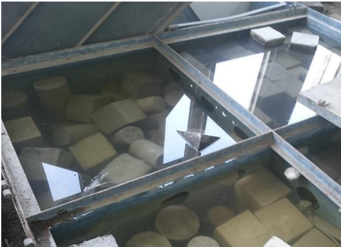
Figure 3.11: Curing of the samples in water tanks
