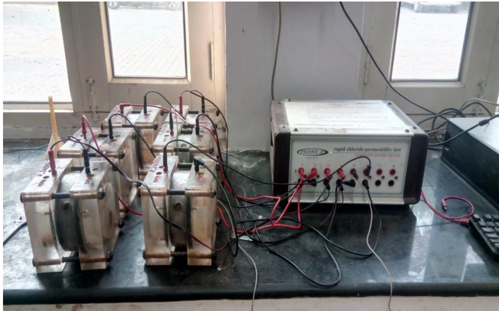
Figure 3.19: Test setup for the rapid chloride permeability test
