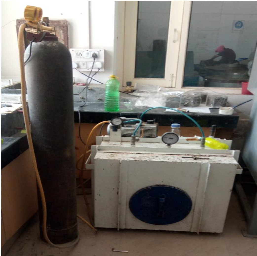
Figure 3.9: Carbonation chamber along with CO 2 cylinder used in this study
