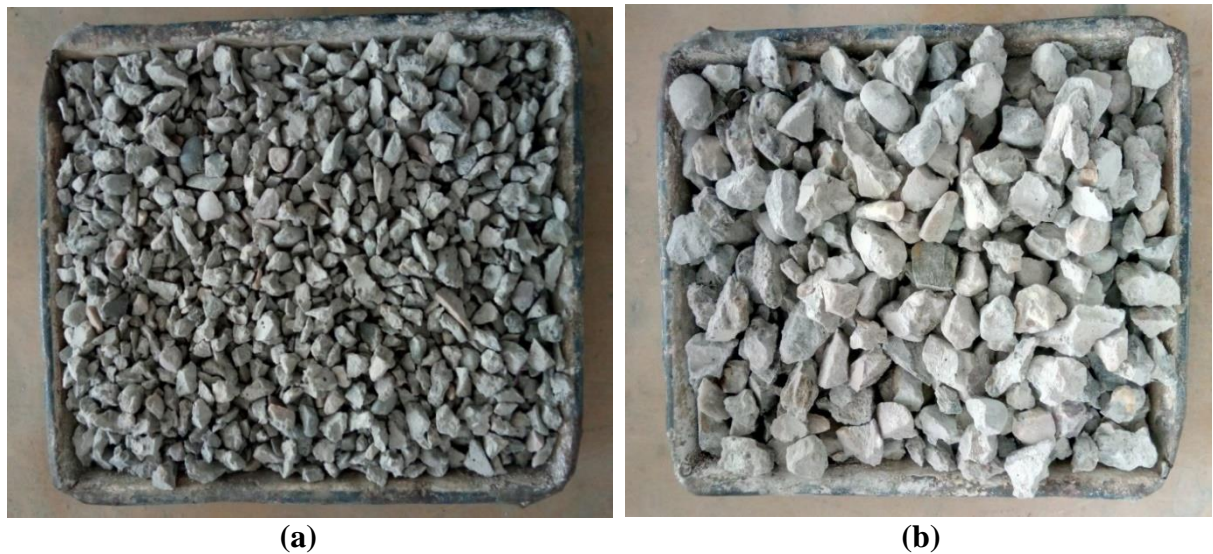
Figure 3.10: Shows the carbonated recycled coarse aggregates of (a) 10 mm maximum size and (b) 20 mm maximum size
