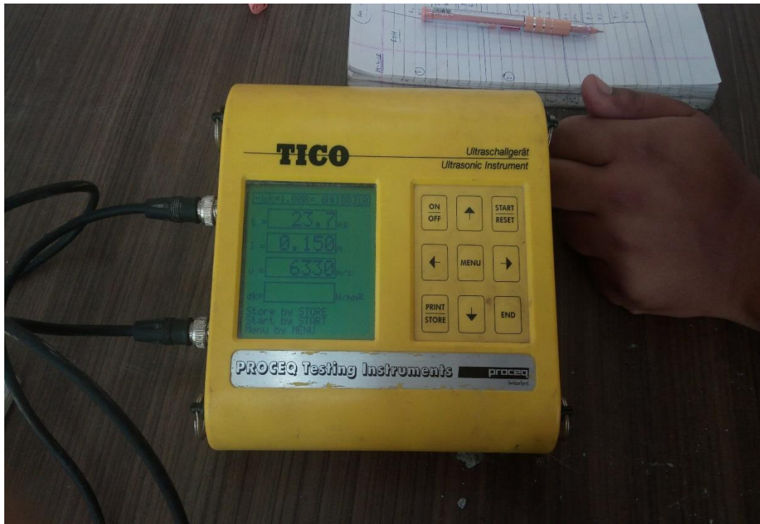
Figure 3.13: Readings shown by Ultrasonic digital instrument
