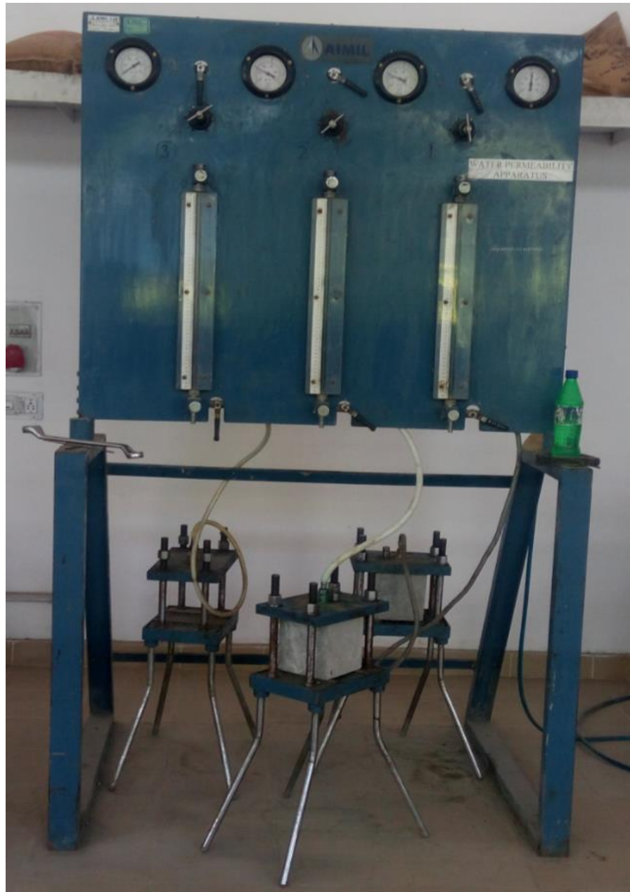
Figure 3.20: Test setup for the water permeability test
