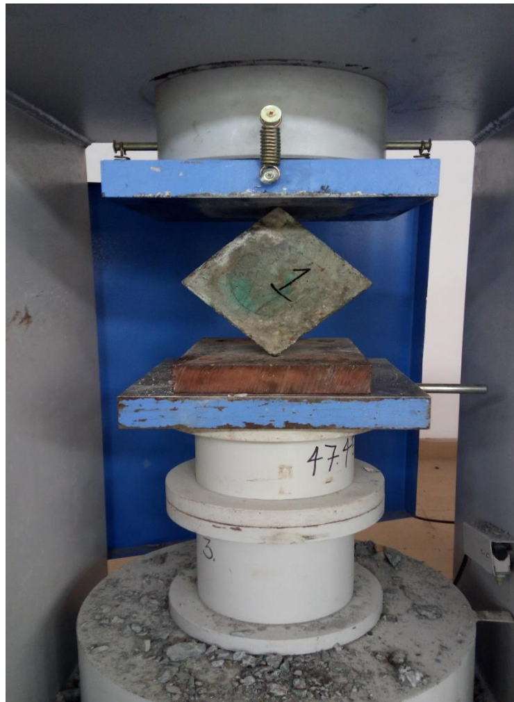
Figure 3.21: Splitting the cube specimen under CTM after removing from the water penetration cell
