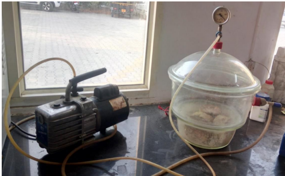
Figure 3.18: Concrete specimens in the vacuum desiccator's bowl
