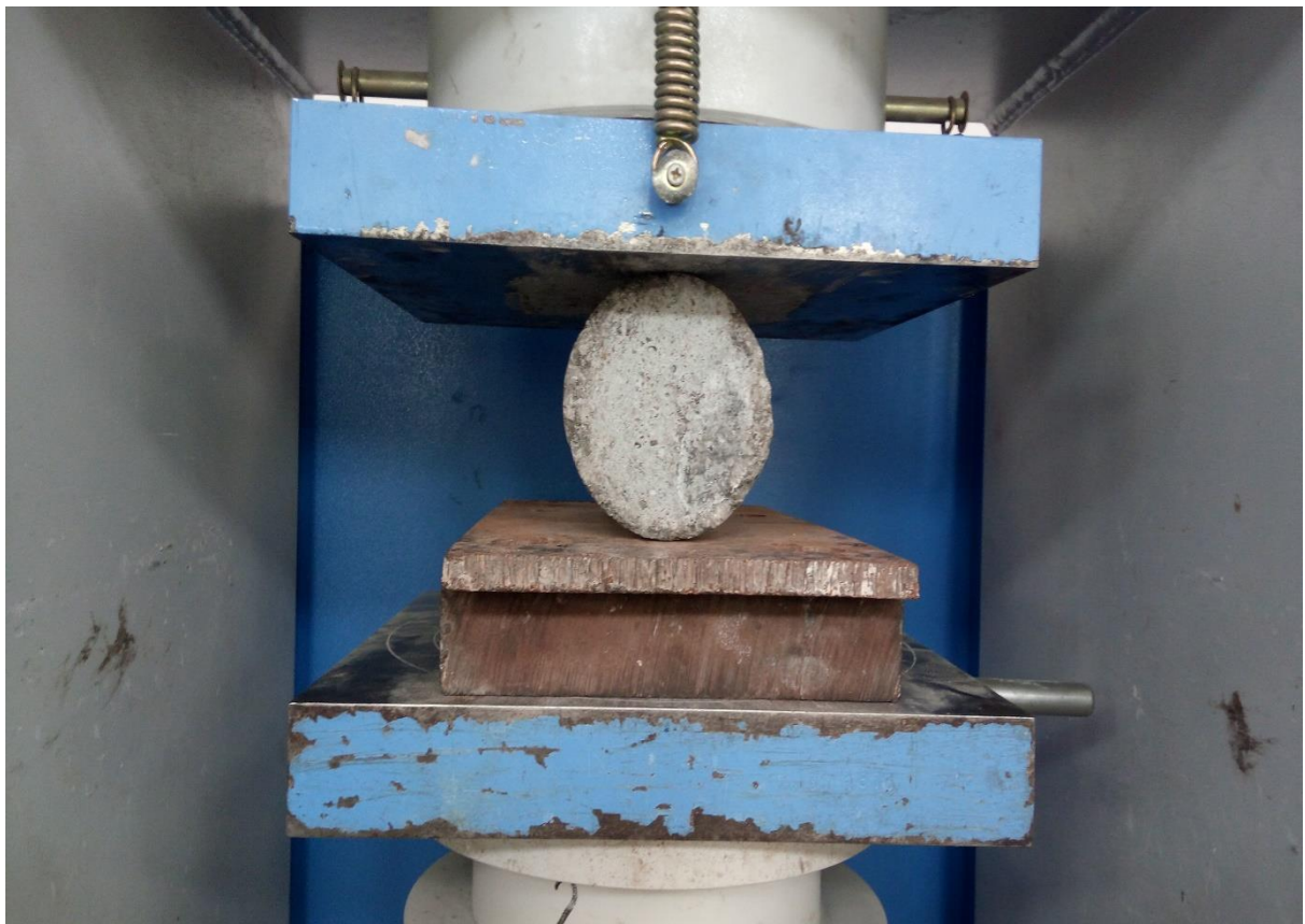
Figure 3.17: Testing of a cylinder for split tensile strength on CTM
