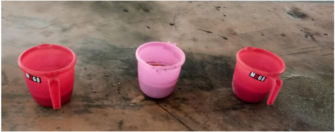
Figure 3.7: Three plastic bathing mugs used, in which recycled coarse aggregates are dipped in an acidic solution
