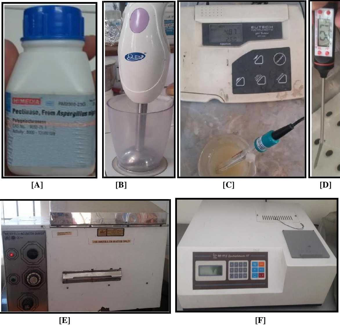
Fig.11: Pectinase enzyme from HIMEDIA [A], Glen hand blender [B], pH meter [C], digital thermometer [D], water bath [E], spectrophotometer [F].
