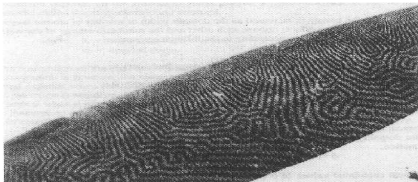
figure 8 (b) Visualization of domains by Faraday rotation with polarized light
