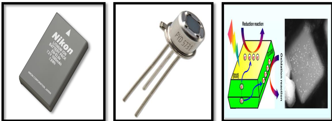
Fig 1.1: Bismuth vanadate used (from left to right) in rechargeable lithium batteries [7], pyroelectric detectors [8], and as a catalyst [9].
