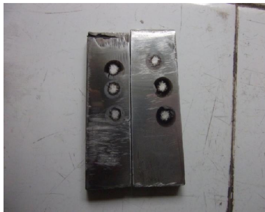
Figure 3.3: Spectroscopic samples of Duplex 2205
