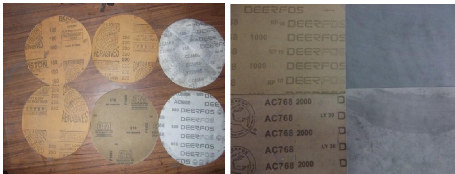
Figure 3.20: Emery papers of different grades
