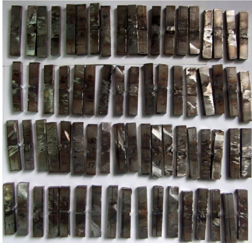
Figure 3.17: Samples prepared for impact test
