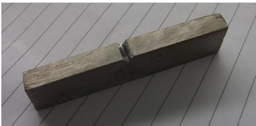
Figure 3.16 Sample with notch angle 45°
