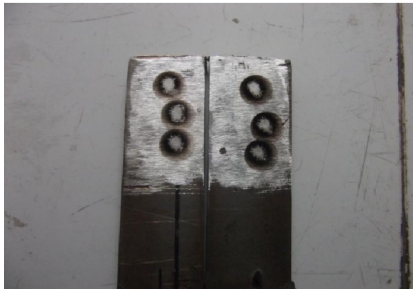
Figure 3.2: Spectroscopic samples of material AISI 316
