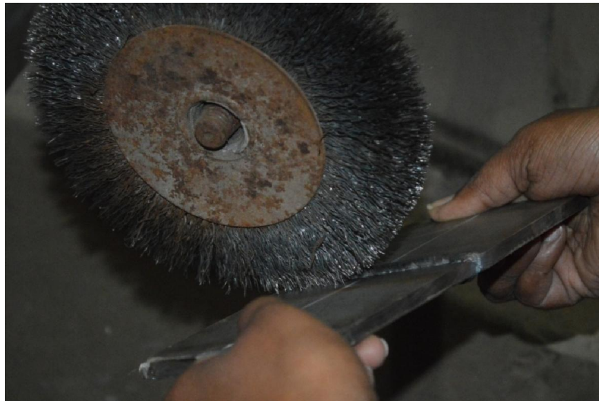
Figure 3.11: Buffing cleans all impurities before and after welding
