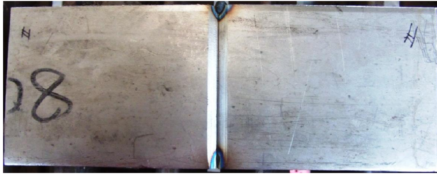
Figure 3.10: Sample with 90° groove
