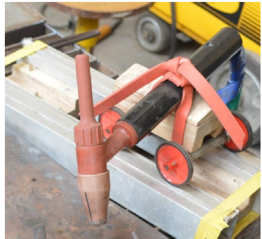
Figure 3.9: Welding cart with the nozzle.
