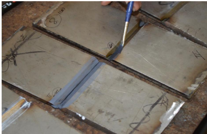
Figure 3.7: Application of flux
