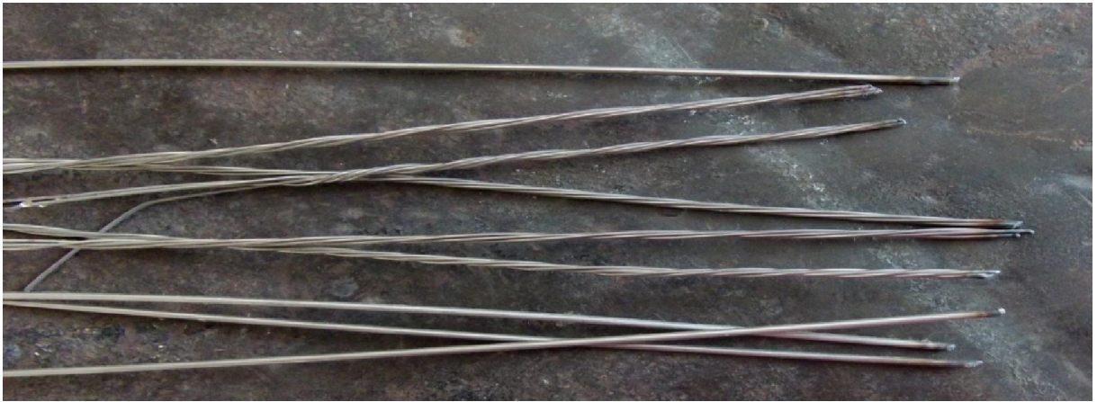
Figure 3.4: Duplex 2205 and AISI 316 Filler Wires
