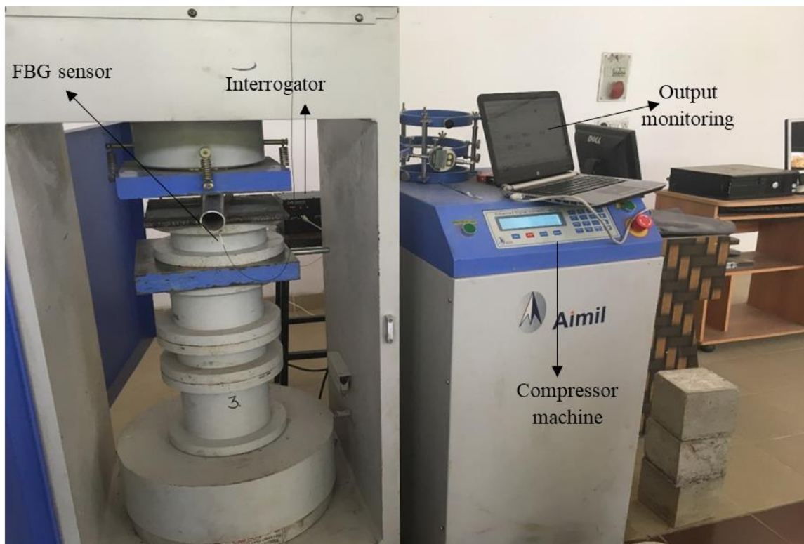
Figure 4.1 Experimental setup for strain monitoring
