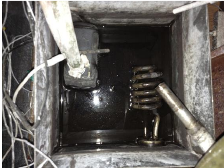
Fig. 3.6: Collecting tank and Heating element
