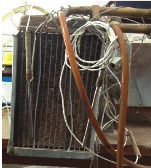
Fig 3.3: Cross flow Heat exchanger
