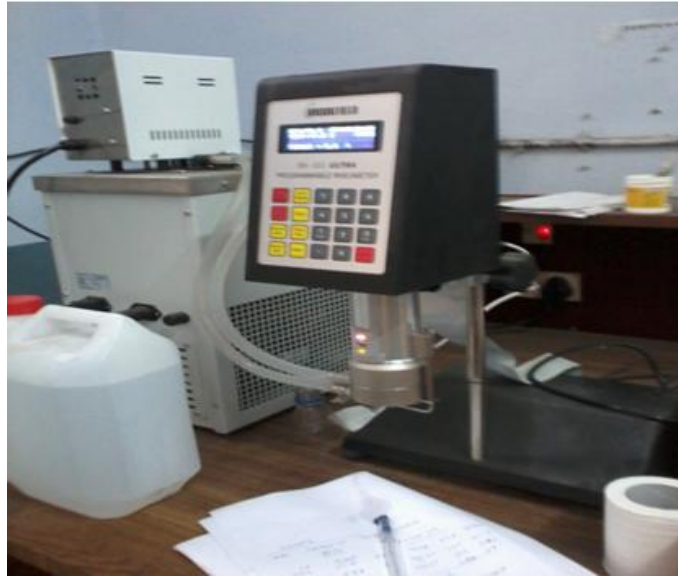
Fig. 3.17: Brookfield DV-III Rheometer.
