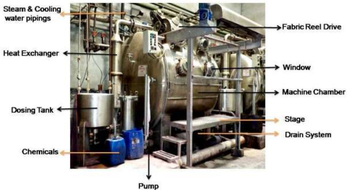
Fig. 4.5(a) Soft-flow machine with components
