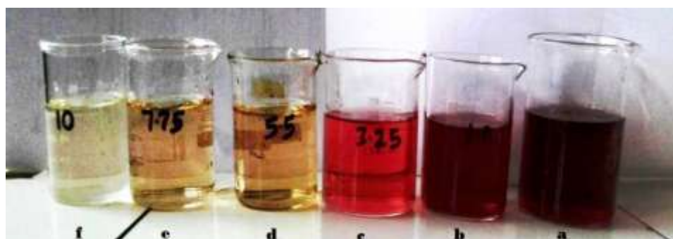
Fig.4.21 Aesthetic representation of original sample (a); Samples at 1 V 1min. (b); 1V 3.25 min. (c); 1 V 5.5 min.(d); 1V 7.75 min. (e) and 1V 10 min. (f)
