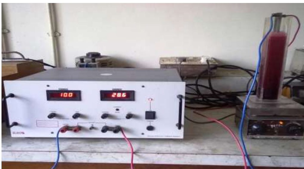
Fig.3.2 Experimental setup for electroflocculation treatment of textile wastewater
