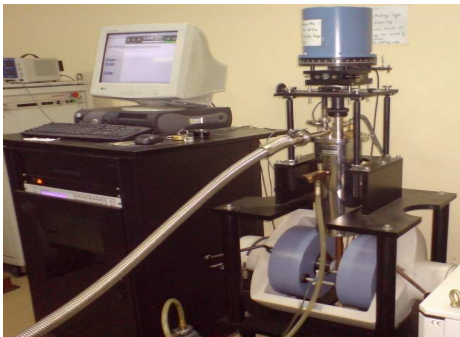
Figure 2.2: Vibrating Sample Magnetometer at NPL, New Delhi.
