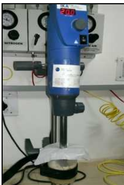
Figure: 3.1 Homogenizer (Photo courtesy: Chemical Engineering Department, Thapar University, Patiala)
