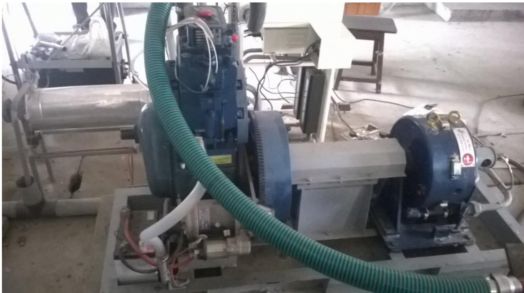
Fig 32 Variable CR dual fuel CI engine setup
