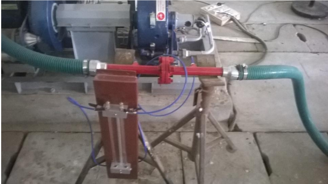
Fig 33 Flowmeter for measuring the volume flow rate of producer gas
