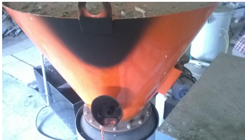
Fig 30 Small/Narrow intake port for air/oxygen intake
