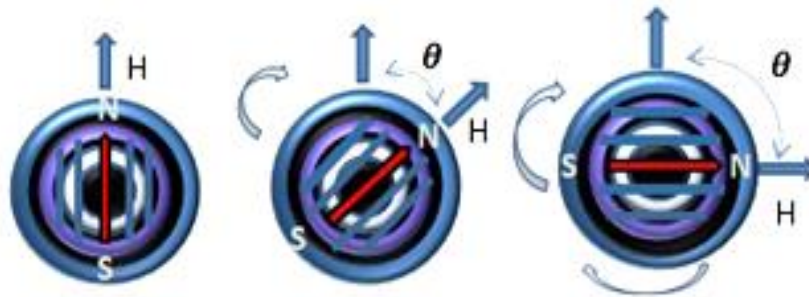
Figure 5 Brownian relaxation of magnetic nanoparticle in the presence of external magnetic field [2].
