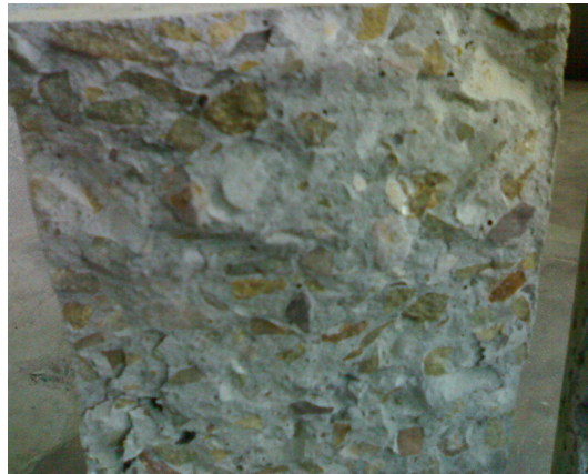
Plate. 4.5. Failure pattern of control concrete
