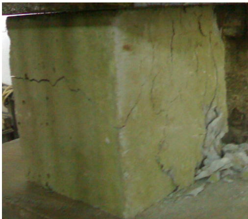
Plate. 4.2 Control concrete cube failure
