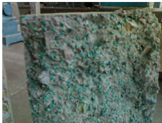
Plate. 4.6. Failure pattern of plastic concrete
