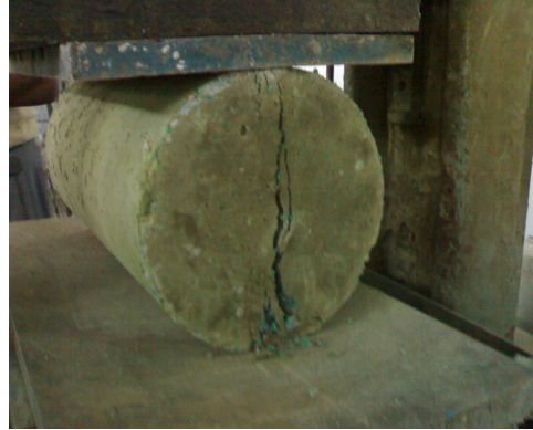
Plate. 4.4. Test set up for conducting split tensile test on cylinders
