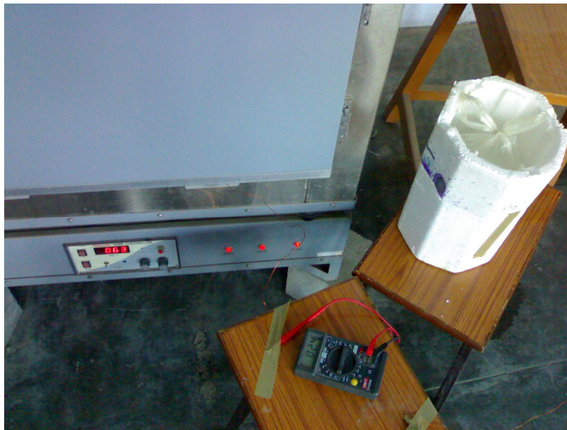
Plate. 3.4. Thermocouple arrangement of concrete cube in oven
