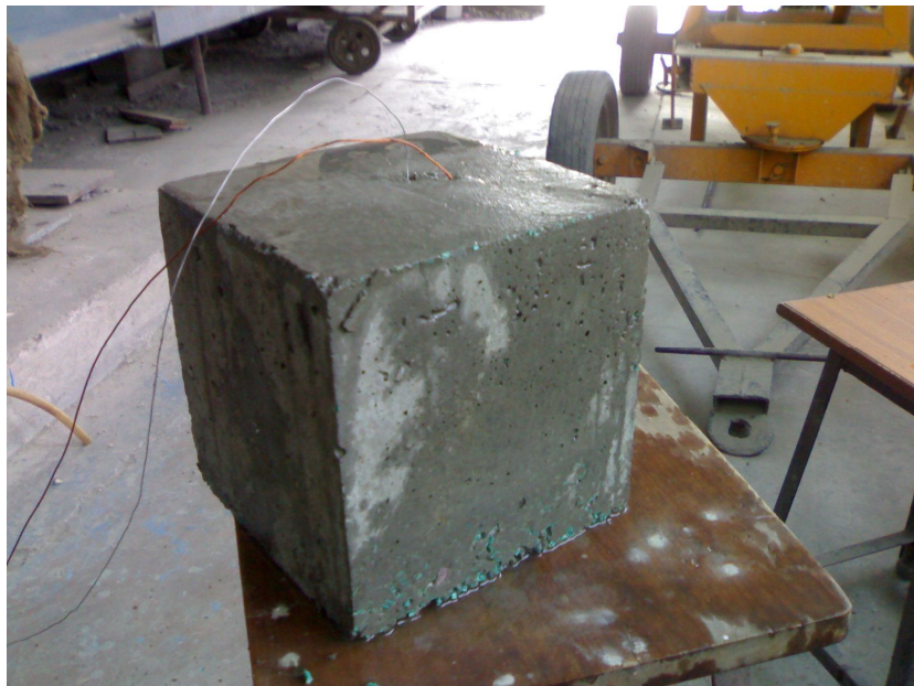
Plate. 3.3. Copper and constantan wires putted into cubes
