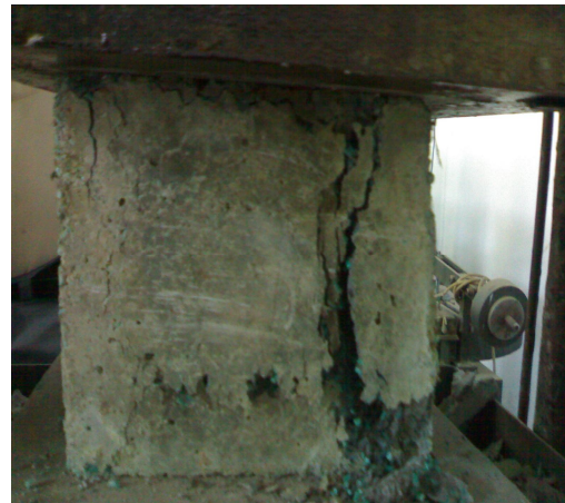
Plate. 4.3 Plastic concrete cube failure
