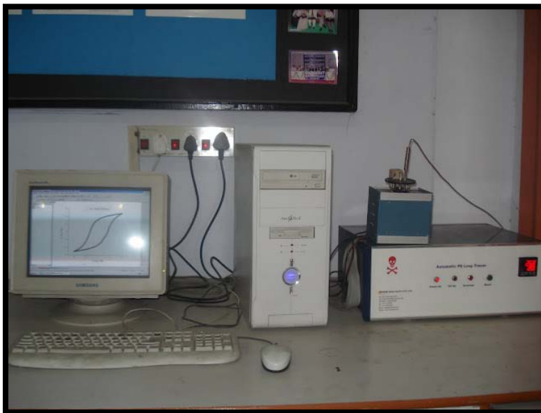
Figure 2.15 P-E Hysteresis Loop Tracer
