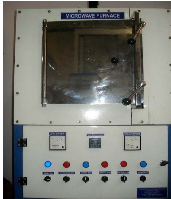
Figure 2.9 Furnace used for Microwave sintering and its various specifications
