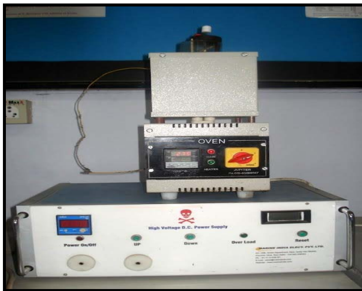
Figure 2.16 Poling set up
