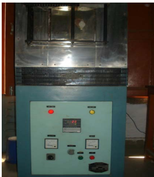
Figure 2.3 Programmable furnace used for calcination and its various specifications
