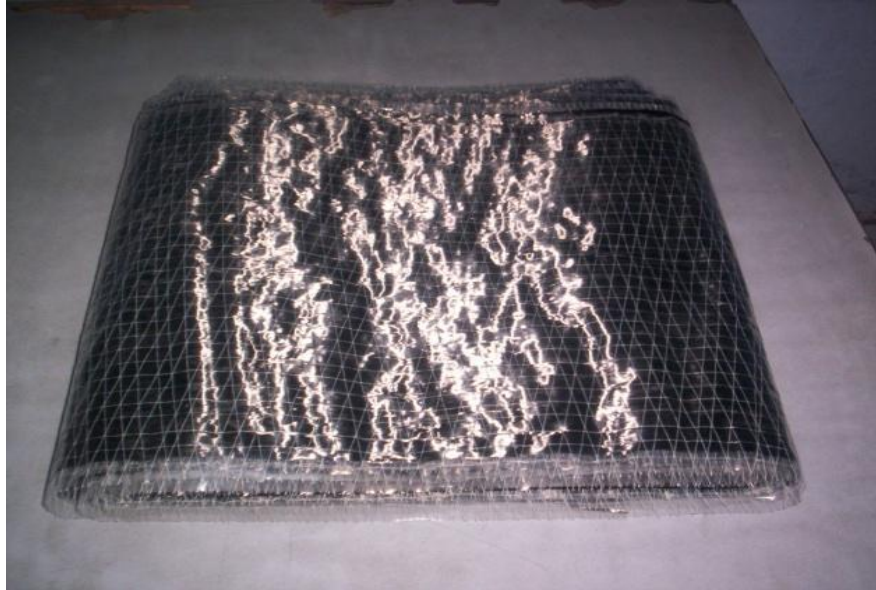
Fig 4.2 CFRP sheet used in the experiment
