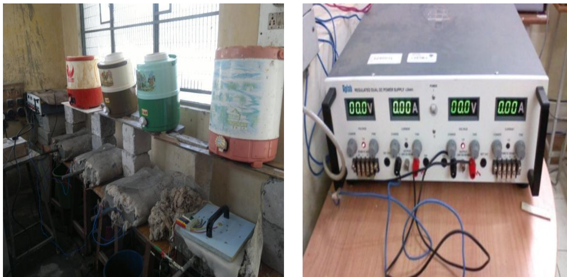
Fig 4.1 Specimens and the Power Supplies Used to Accelerate Corrosion
