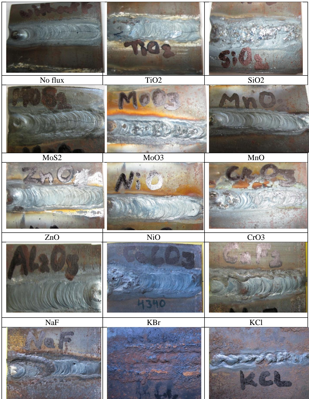
Figure 3.32: Macrographs show the bead appearance for AISI 4340 steel at 125 A with and without flux/compound
