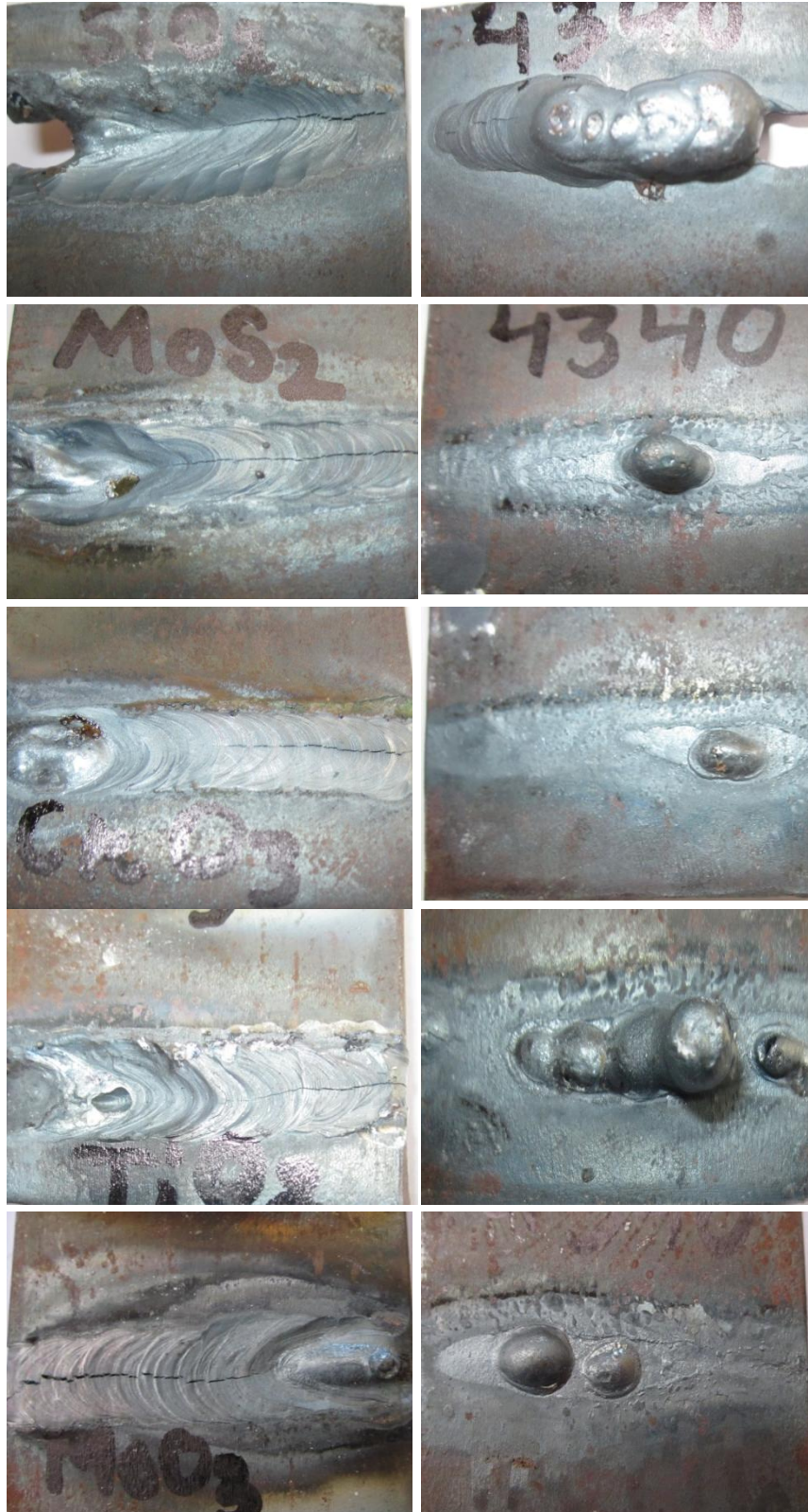
Figure 3.47: Macrographs shows the bead appearance for AISI 4340 steel at 125 A with 5 different fluxes and with Ar+5% H 2 shielding at flow rate of 10 L/min.
