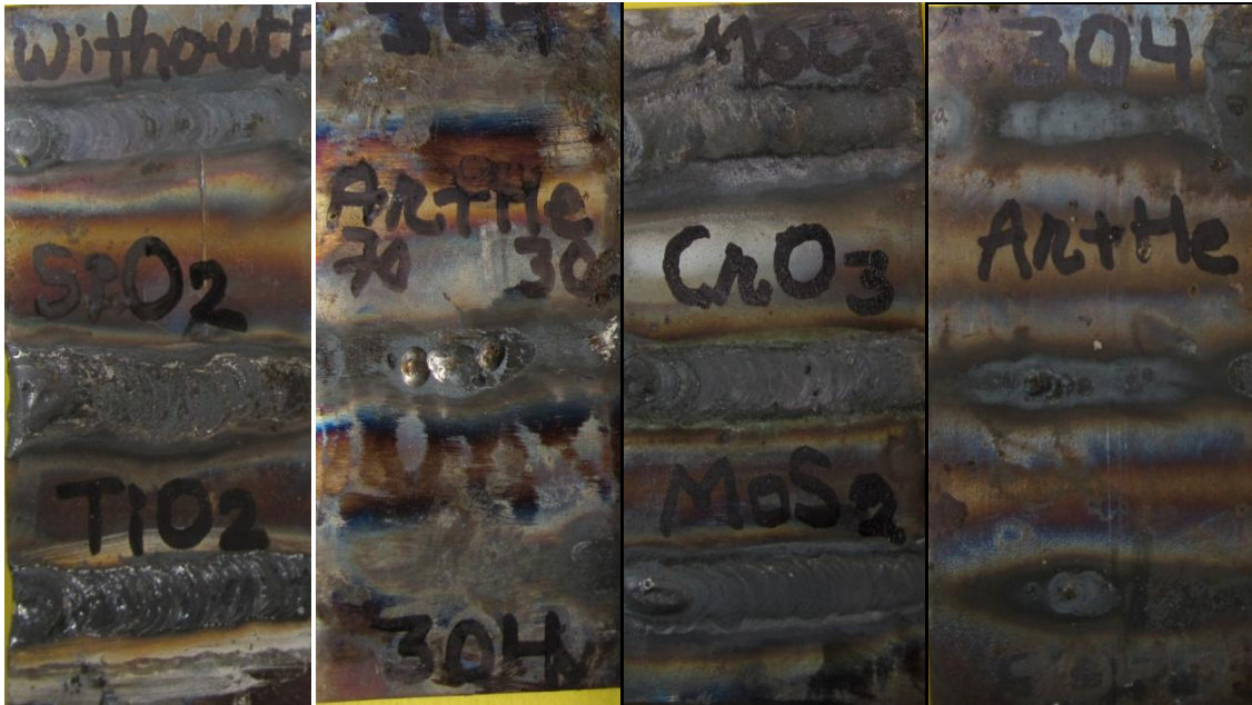
Figure 3.54: Weld bead appearance (top, bottom surface) of A-TIG with five different fluxes for AISI 304 workpiece (100 A, Ar 70 % + He 30 %, flow rate 10 L/min)
