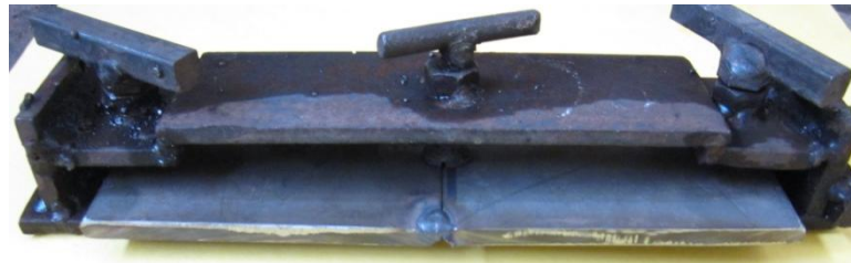
Figure 4.9 Tacked workpieces in jig
