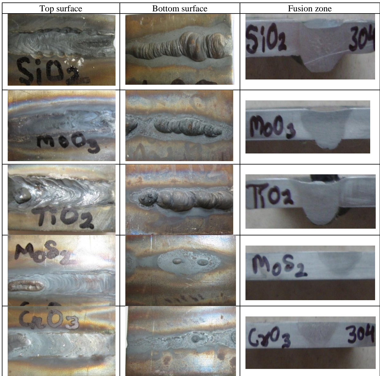
Figure 3.38: Weld bead appearance (top, bottom surface) and photographic view of the fusion zone after A-TIG with five different fluxes for AISI 304 workpiece (125 A, Ar + 5% H 2 , flow rate 10 L/min)
