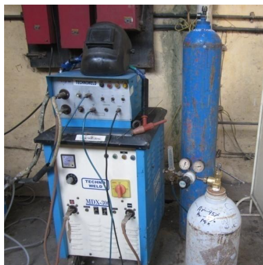
Figure 4.10: A-TIG welding setup
