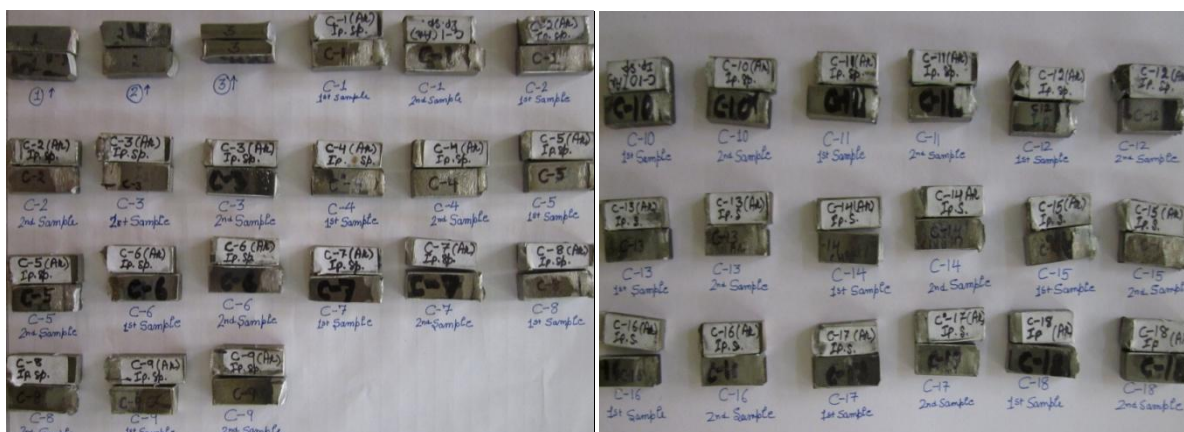
Figure 4.32: Broken specimens after toughness test of A-TIG welding joint of AISI 304 under Ar shielding
