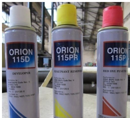
Figure 4.18: Cleaner, penetrant and developer used for DPT
