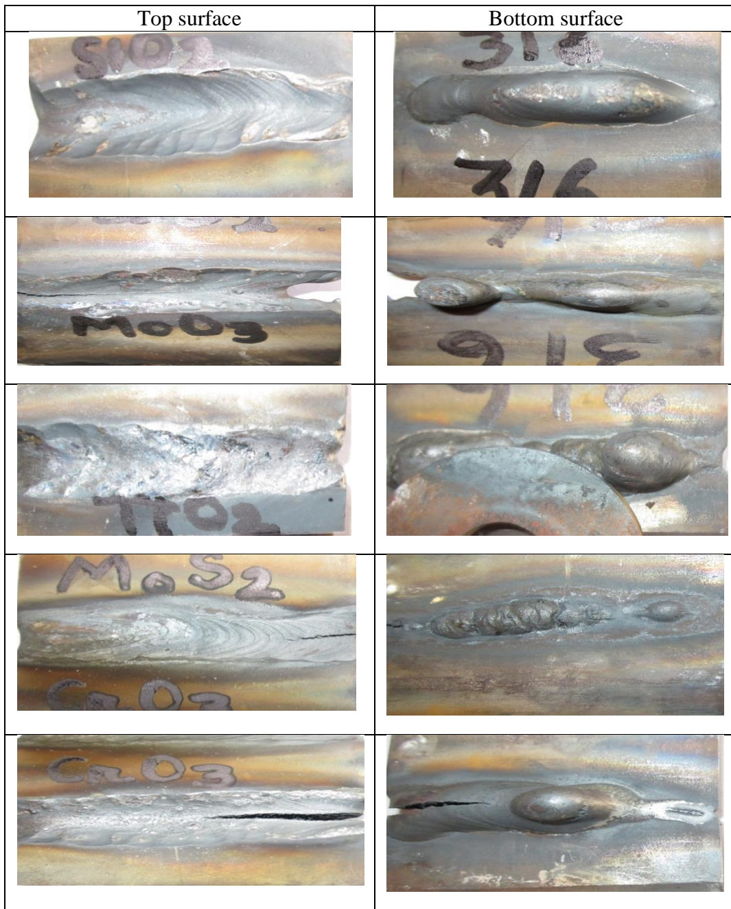
Figure 3.41: Macrographs shows the bead appearance for AISI 316 steel at 125 A with 5 different fluxes and with Ar+H 2 5% shielding at flow rate of 10 L/min.
