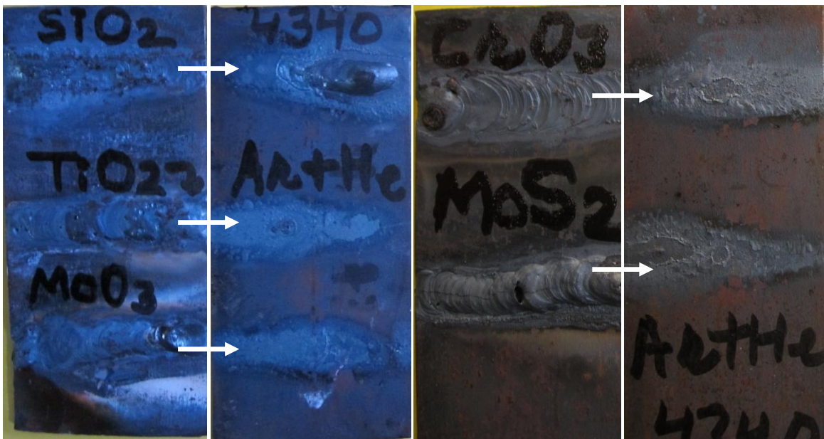
Figure 3.53: Weld bead appearance (top, bottom surface) of A-TIG with five different fluxes for AISI 4340 workpiece (125 A, Ar 70 % + He 30 %, flow rate 10 L/min)
