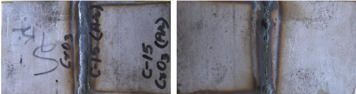
Figure 4.35: Top and backside of Sample-15 (C-15) welded under Ar shielding with CrO 3
