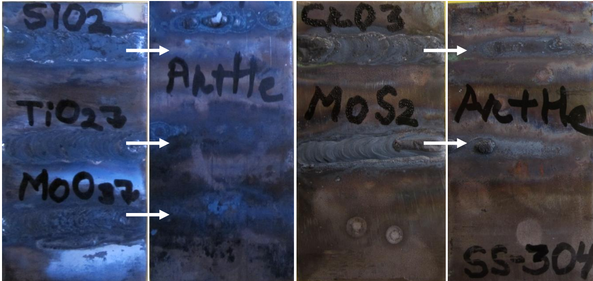
Figure 3.50: Weld bead appearance (top, bottom surface) of A-TIG with five different fluxes for AISI 304 workpiece (125 A, Ar 70 % + He 30 %, flow rate 10 L/min)
