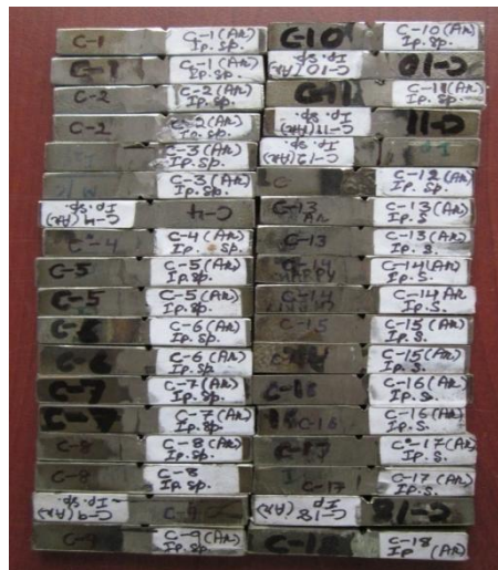
Figure 4.31: Toughness specimens after toughness test of A-TIG welding joint of AISI 304 under Ar shielding
