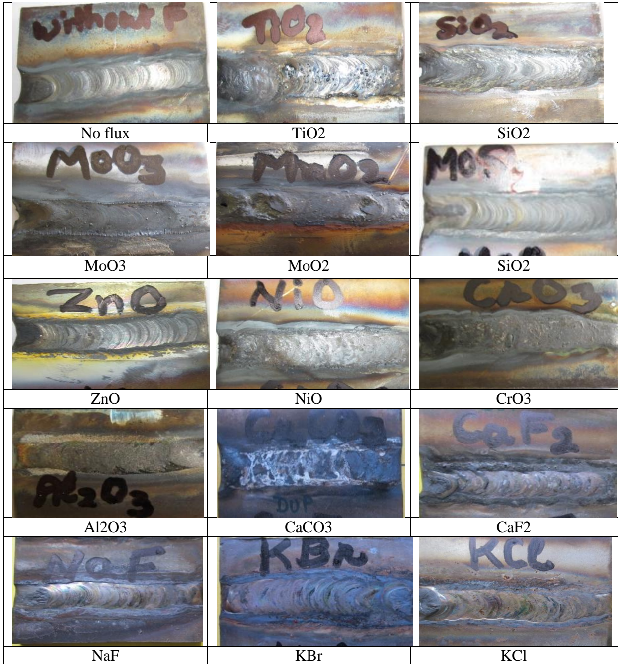
Figure 3.29: Macrographs shows bead appearance for DUPLEX 2205 steel at 125 A with and without flux/compound
