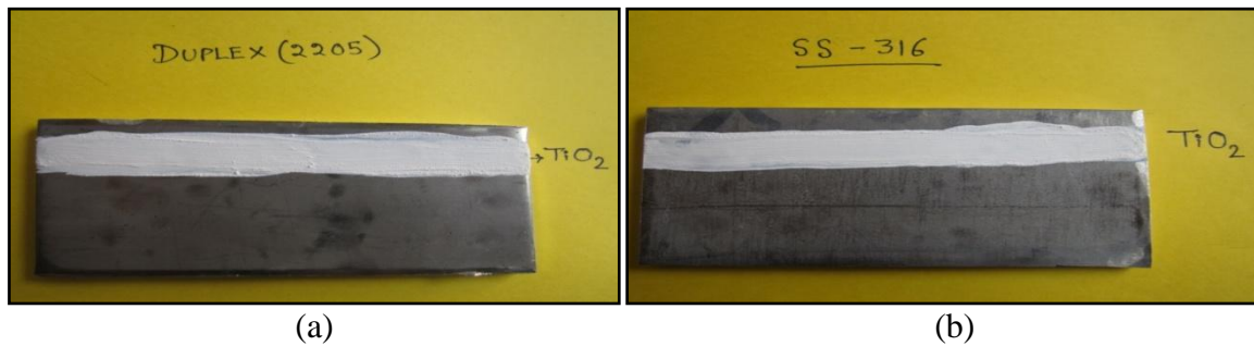
Figure 3.3: (a) Duplex 2205 with \text{TiO}_2 flux coating, (b) AISI 316 plate with \text{TiO}_2 flux coating
