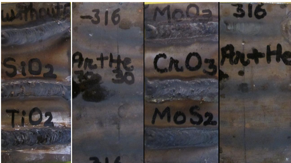
Figure 3.55: Weld bead appearance (top, bottom surface) of A-TIG with five different fluxes for AISI 316 workpiece (100 A, Ar 70 % + He 30 %, flow rate 10 L/min)
