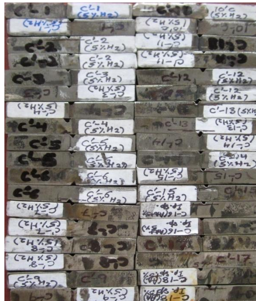
Figure 4.36: Toughness specimens after toughness test of A-TIG welding joint of AISI 304 under Ar+5%H 2 shielding
