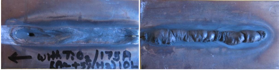
Figure 4.1: Macrograph showing weld bead appearance of A-TIG welding on AISI 304 at 175 A, with Ar+5%H 2 as shielding at a flow rate of 10 L/min at welding speed of 3 mm/sec.
