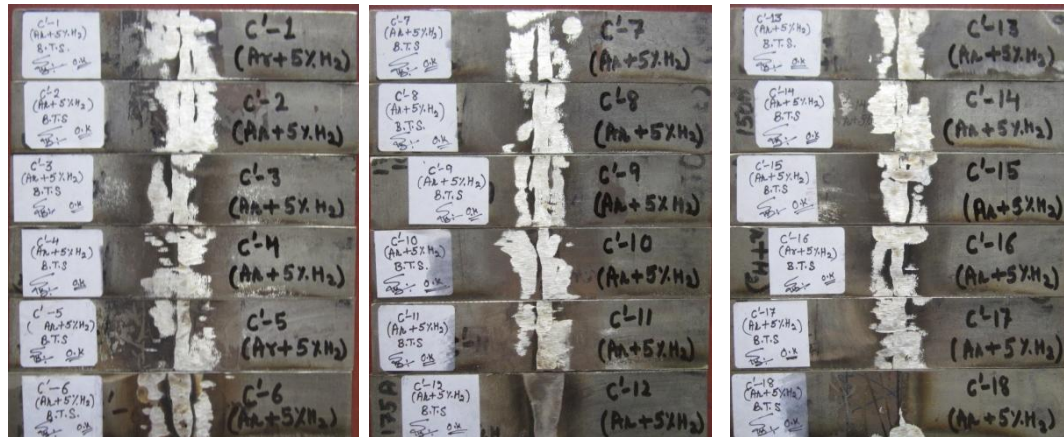
Figure 4.26: Face bend specimen of A-TIG welding of AISI 304 under Ar+5% H_2 shielding
