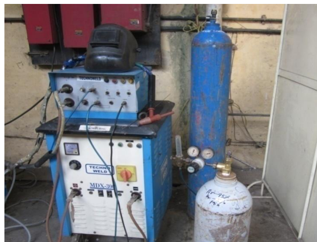
Figure 3.4: TIG Welding Set-up
