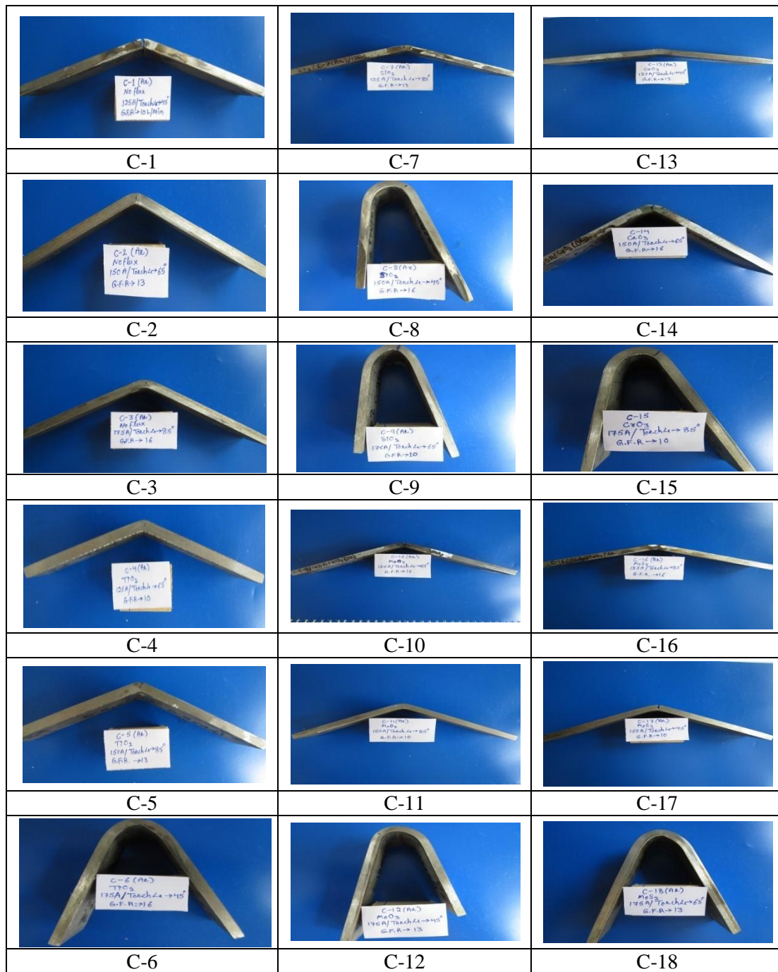
Figure 4.24: Front view of bend test specimen of A-TIG welding of AISI 304 under Ar shielding
