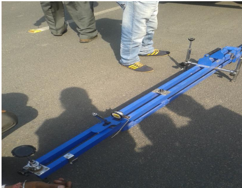
Plate 3.7: View of Benkelman Deflection Beam
