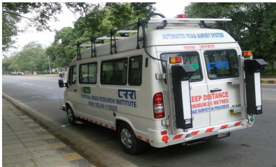
Plate3.5: Automated Road Survey System Being Used on the Project Road for Measurement of Pavement Surface Roughness
