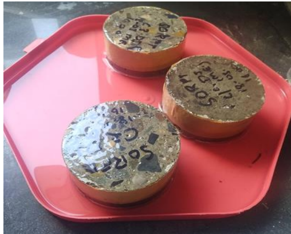
Fig 3.15: Sorptivity Test Setup
