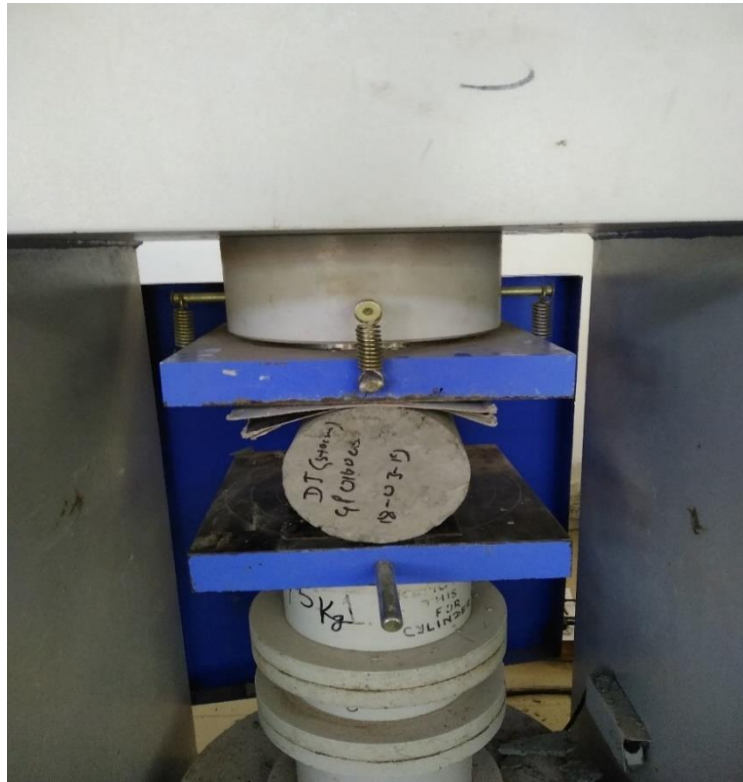
Fig 3.14: Split Tensile Strength Test Setup
