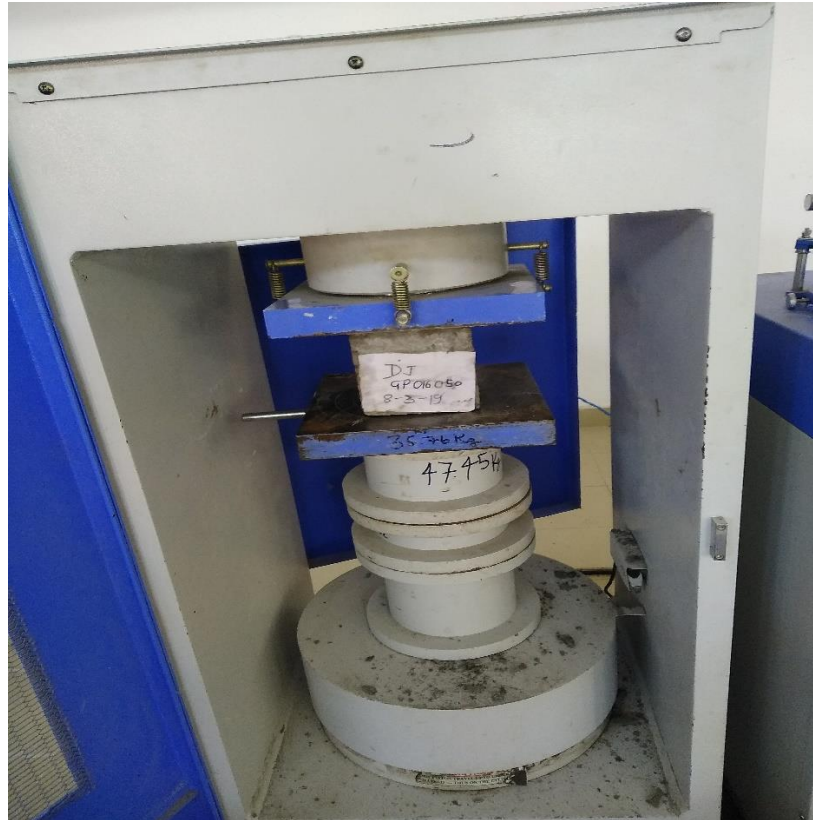
Fig 3.13: Compressive Strength Test Setup
