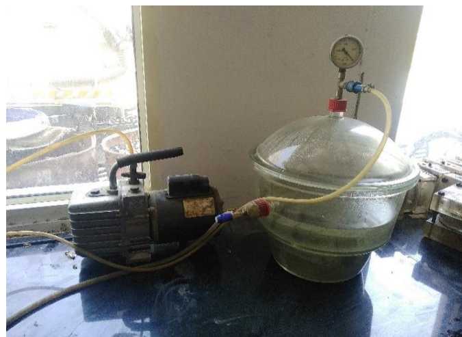
Fig 3.16: Vacuum Pump & Desiccator
