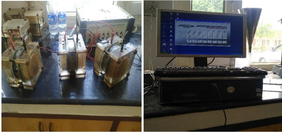
Fig 3.17: RCPT Test Setup
