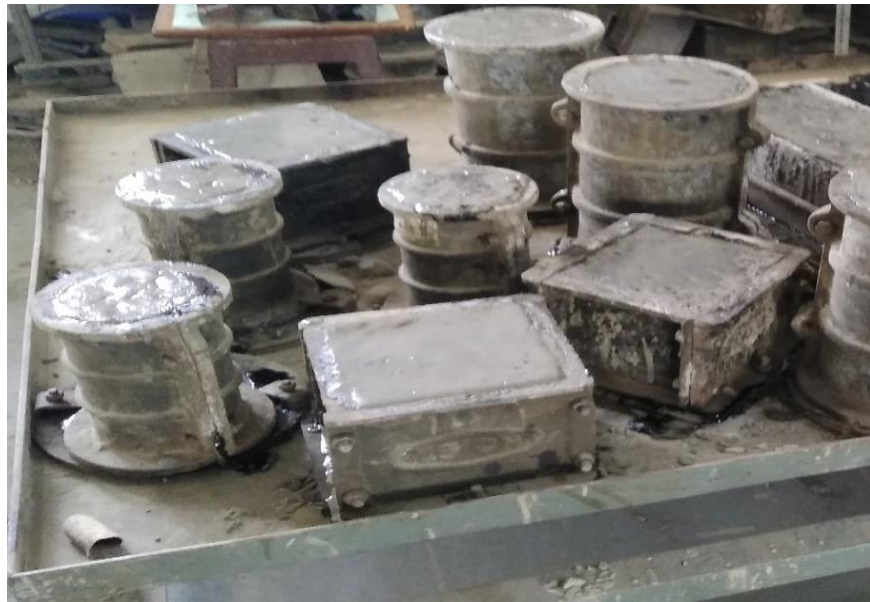
Fig 3.12: Cast Molds containing Geopolymer Concrete
