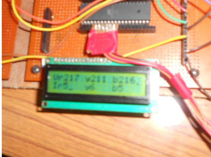
Fig. 4.8 LCD display showing the motor voltage and current
