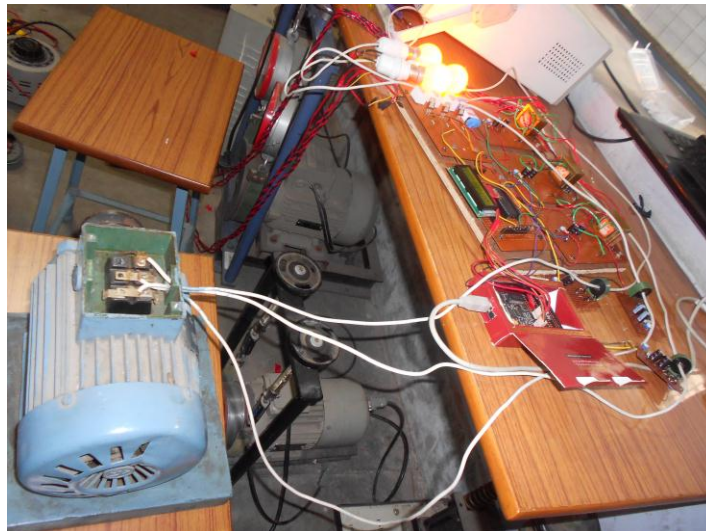
Fig. 4.7 Three Phase Induction motor running with protection system
