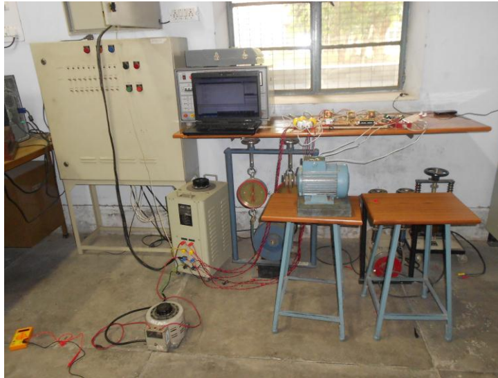
Fig. 4.6 Protection setup of Three Phase Induction motor
