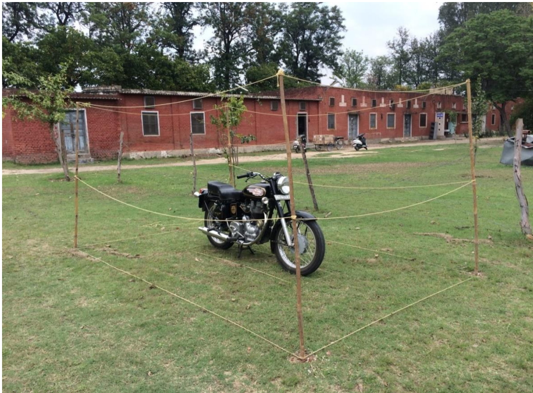
Fig.5.1 Set-up for Measuring the Acoustic Power
