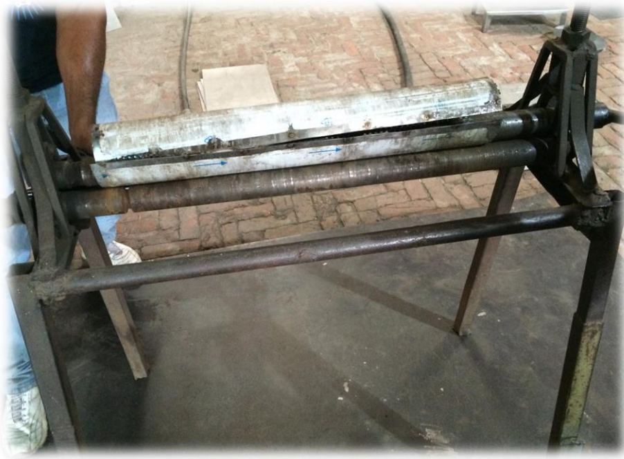
Fig. 4.15 Sheets rolled in bending machine
