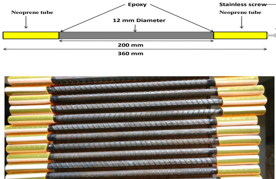
Figure 5.2 Line diagram and actual prepared TMT steel bars
