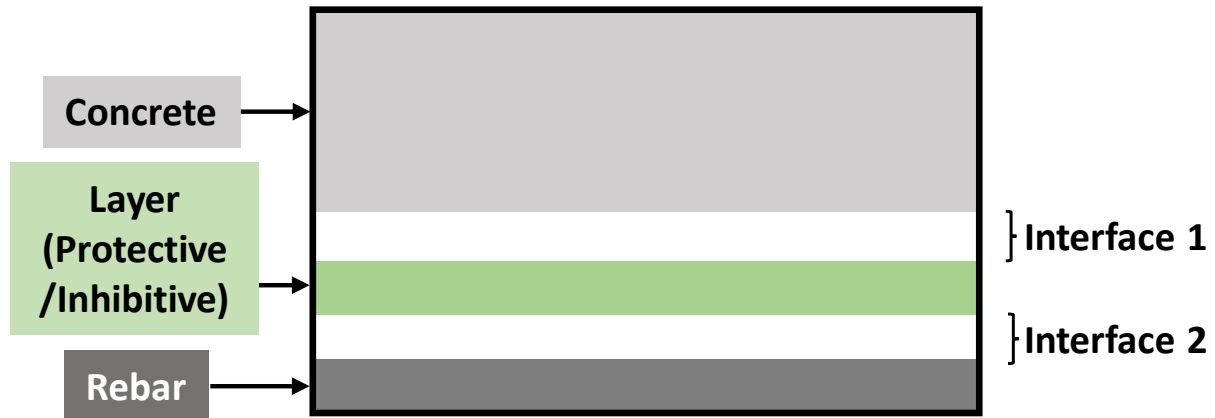
Figure 5.13 Schematic representation of steel-concrete interfaces
