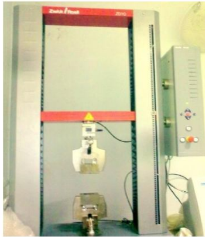
Fig. 4.3.1: UTM testing machine
