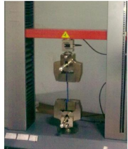
Fig. 4.3.2: Specimen in jaws
