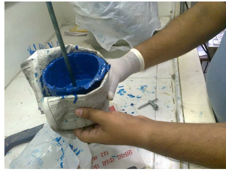
Fig. 4.2.3: Mixing of PET fiber Epoxy solution
