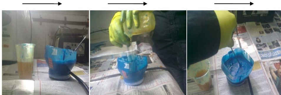
Fig. 4.2.4: Mixing of hardener to the solution
