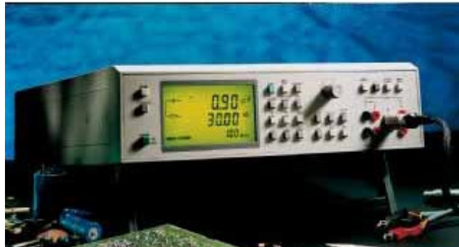
Fig. 2.8 Programmable automatic RCL meter [FLUKE PM6306] used for dielectric studies.
