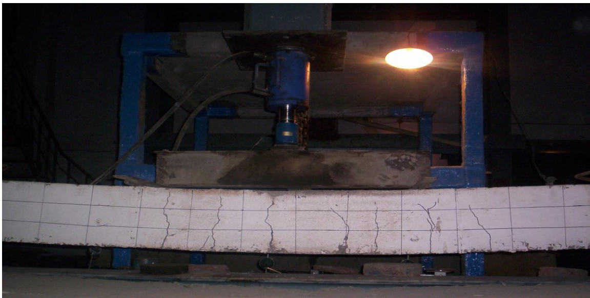
Fig 3.5 Deflected beam & cracks in the central region of the beam
