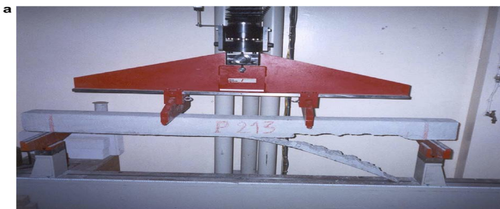
Fig. 2.8 Repaired beam failure by peeling off.(Benjeddou et al, 2006)
