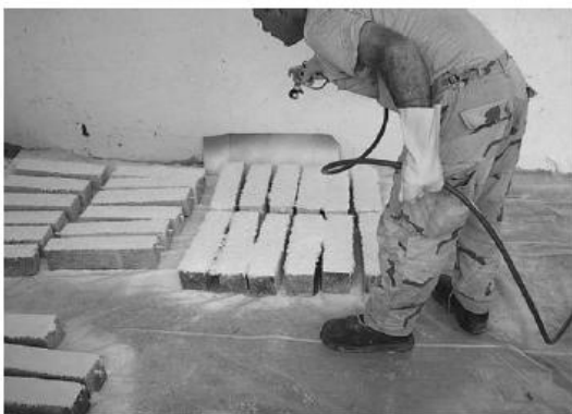
Fig 2.17 Method of applying SFRP
