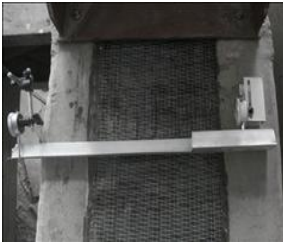
Fig 3.8 Dial gauges for measuring slippage
