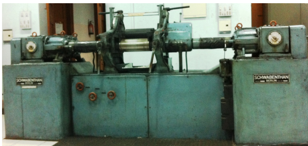
Figure 4.2. Two-roll mill used for preparing blends
