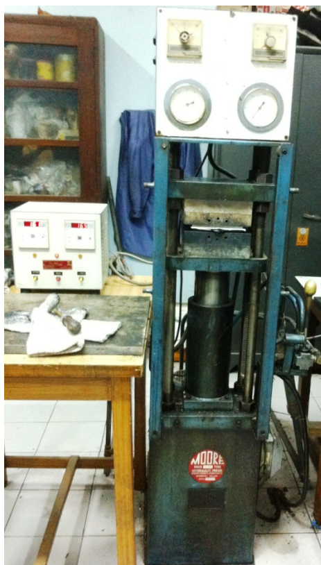
Figure 4.3. Compression moulding machine (hot press) used for preparing film samples
