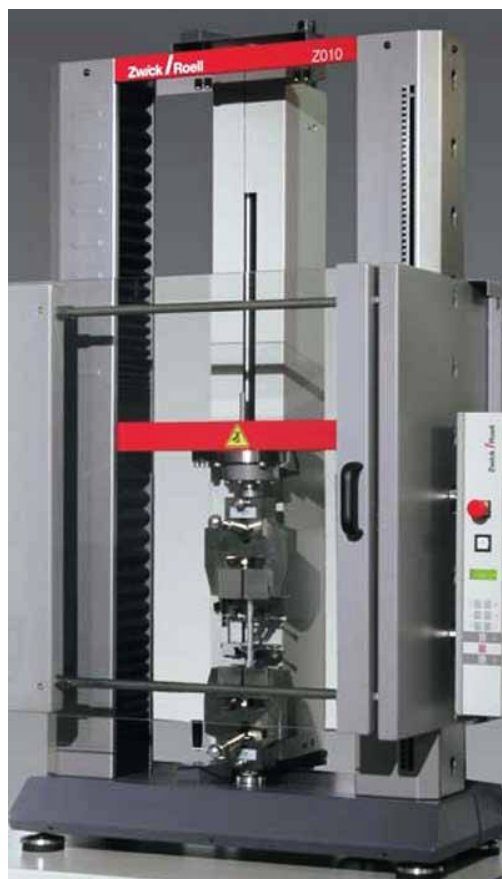
Figure 3.2. Zwick Roell universal testing machine used for performing mechanical testing of the samples
