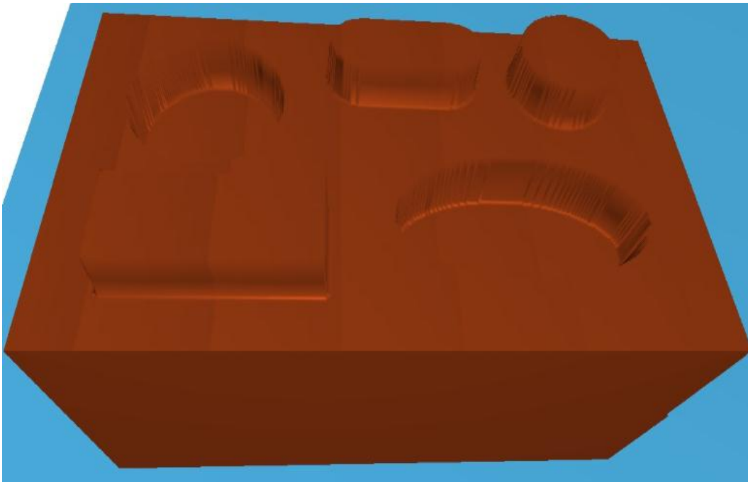
Figure4.15: Pencil Cutting Path for Cavity_Protusion Modal
