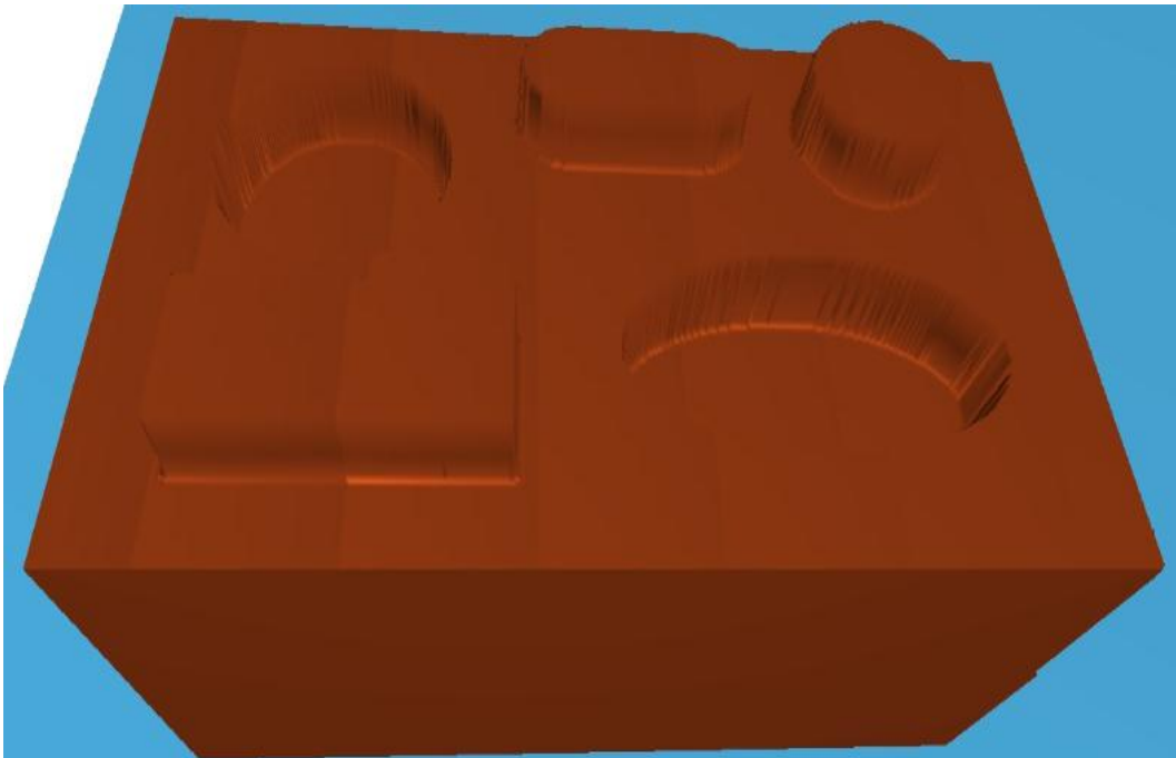
Figure4.11: Cavity_ Protrusion _Modal without Pencil Cutting
