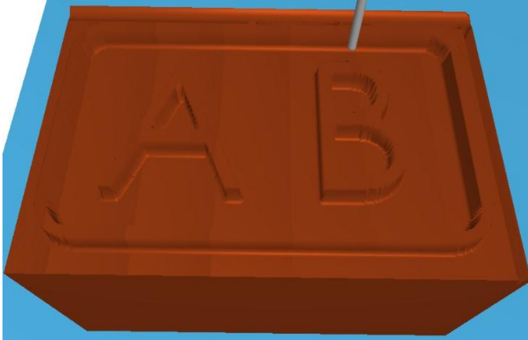
Figure4.5: Pencil Cutting for 0.5 Side Step
