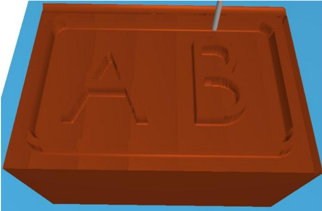
Figure4.7: Pencil Cutting for 0.3 Side Step
