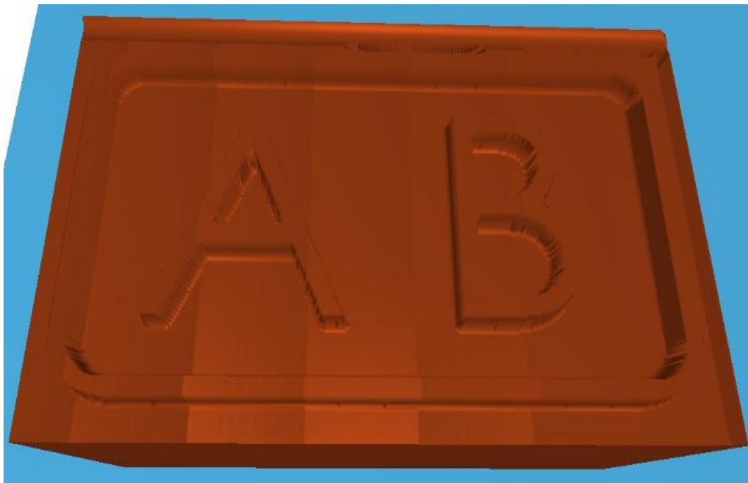
Figure4.6: Pencil Cutting for 0.4 Side Step
