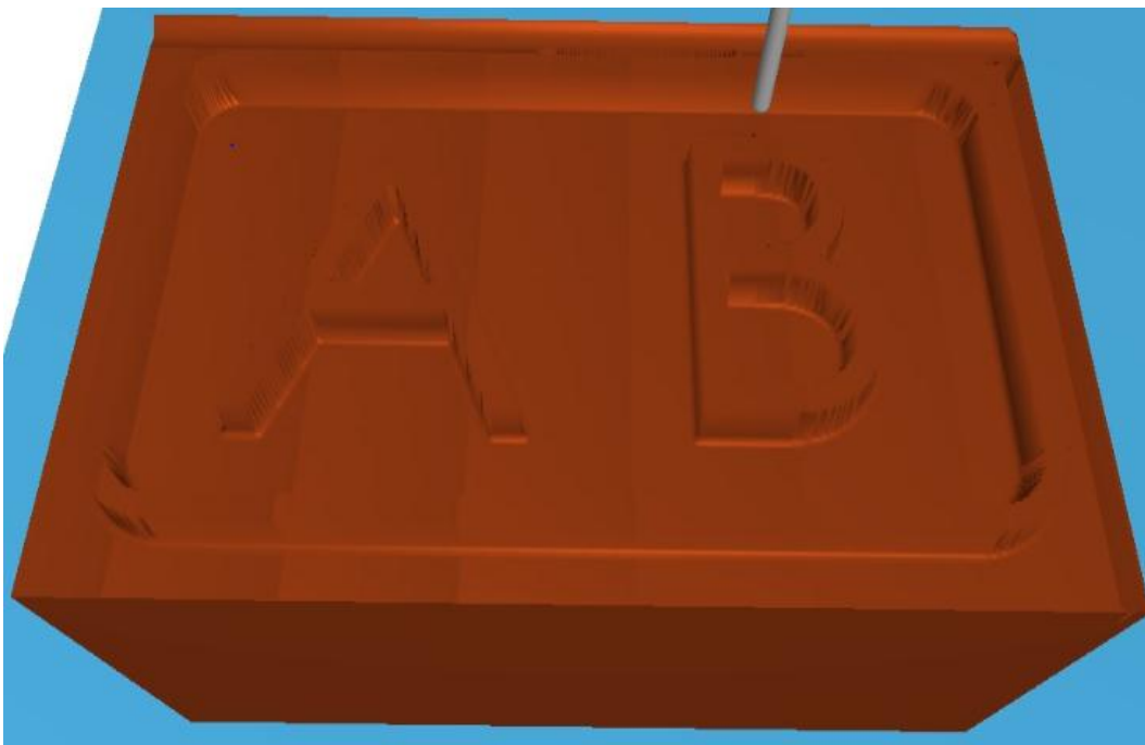
Figure4.8: Pencil Cutting for 0.2 Side Step
