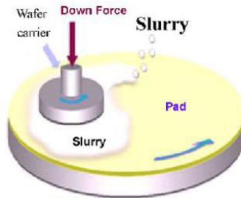
Figure 1.6: Chemo-mechanical polishing process [Nanz et al., 1995].
