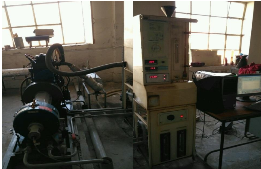
Figure 3.10: Variable compression ratio engine
