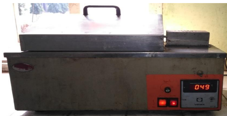
Figure 3.5: Water bath shaker
