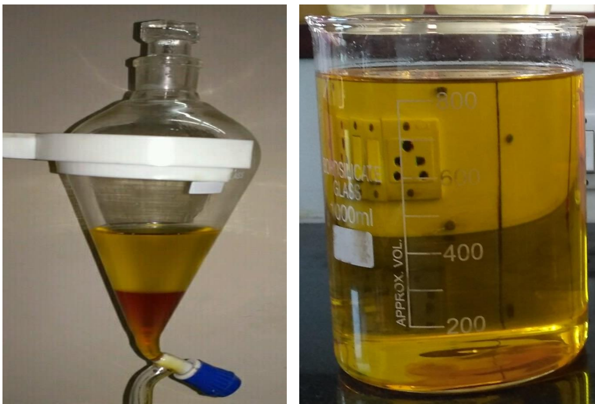
(a) (b) Figure 3.2: (a) Different phases of methyl ester, (b) Safflower biodiesel
