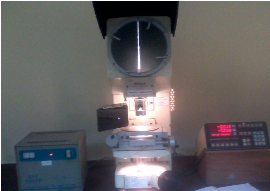
Figure 3.2: Profile projector [Metrology lab, Thapar University]
