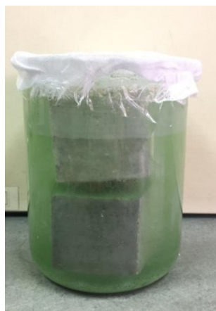
Fig 3.3 Curing of cubes with cyanobacterial cells
