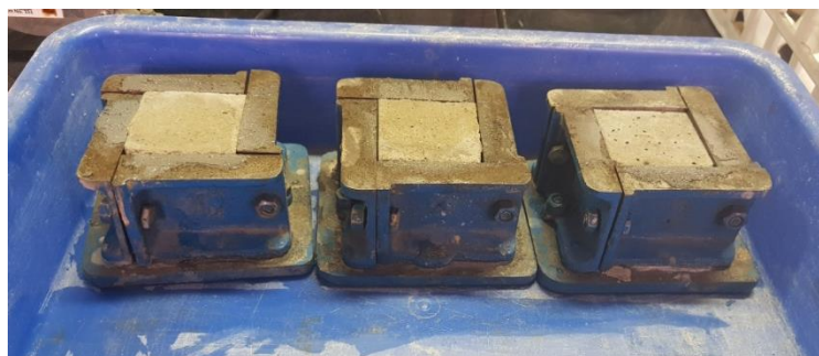
Fig 3.6 Cement mortar cubes ready for demoulding
