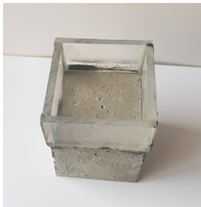
Fig 3.4 Reservoir made on cube for ponding
