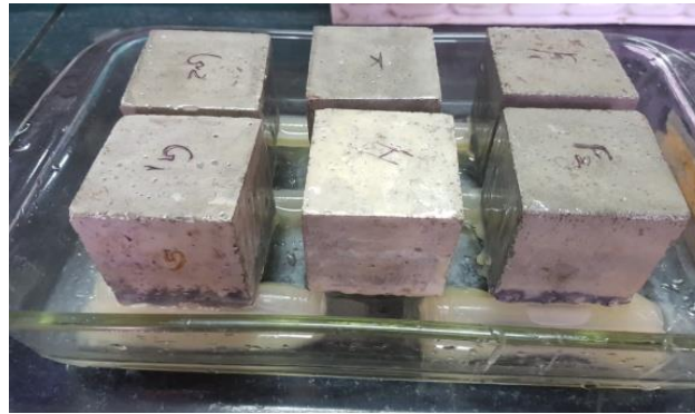
Fig 3.7 Water absorption test conducted on mortar cube specimen
