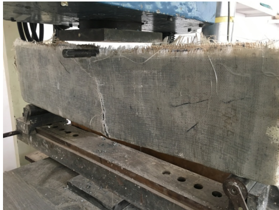
Figure 4. 17 : Showing crack pattern at ultimate load of beam UW-B2 beam.
