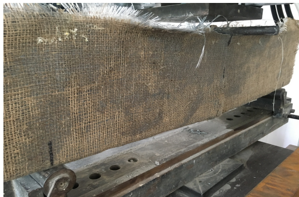
Figure 4. 21 : Showing no de-bonding of FRP even at ultimate failure load.
