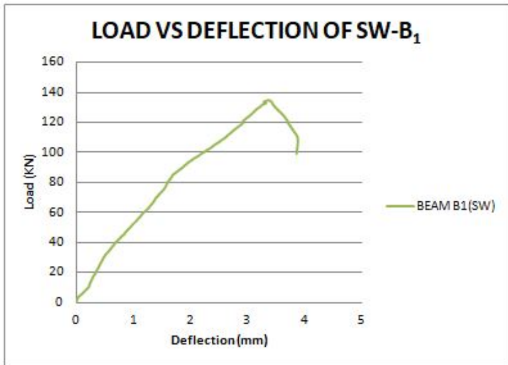
Figure 4. 5 : Graph showing load-deflection behaviour of SW-B1 beam.
