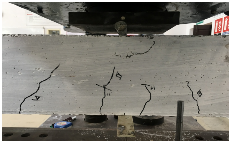
Figure 4. 1 : Showing crack pattern at 60% of failure load
