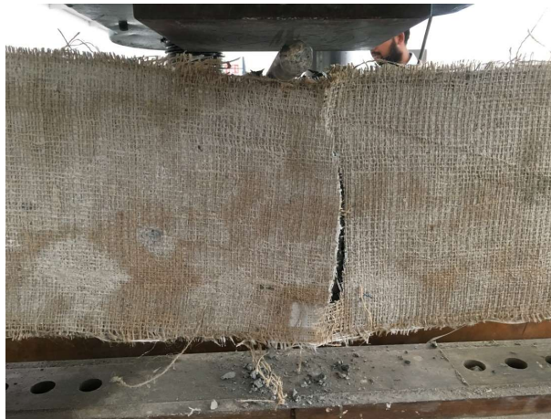
Figure 4. 11 : Showing de-bonding of FRP at bottom of the beam.
