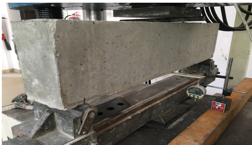
Figure 3. 4 : Testing arrangement for the test beams in UTM
