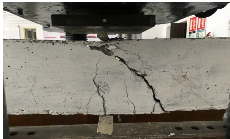
Figure 4. 2 : Showing ultimate failure crack of the control beam.
