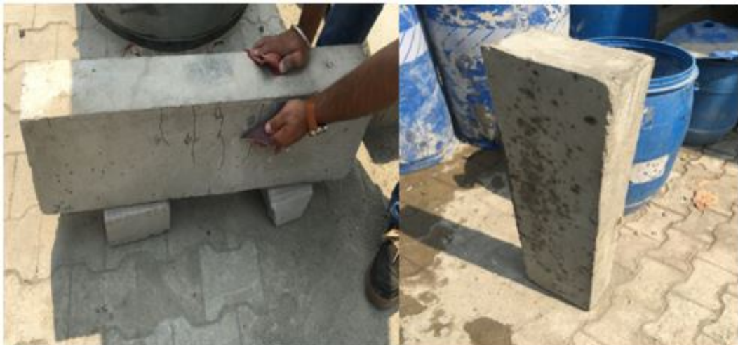
Figure 3. 5 : Showing rubbing of beam surface with sand paper and then washing with water jet.
