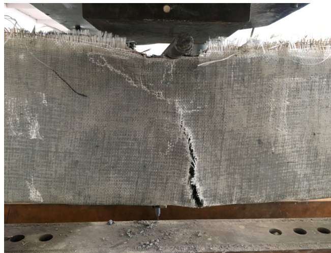
Figure 4. 18 : Showing clear view of the only flexure crack at ultimate load of UW-B2 beam.
