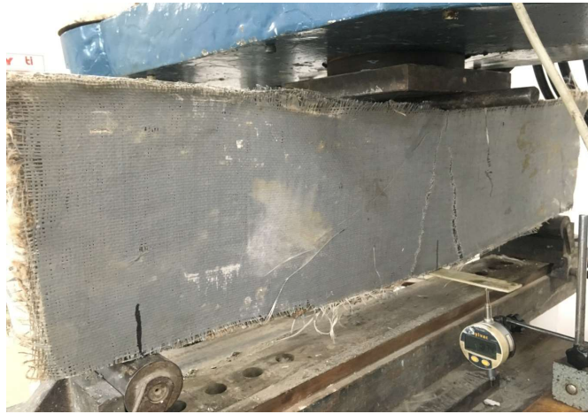
Figure 4. 7 : Showing flexural failure of SW-B2 beam.
