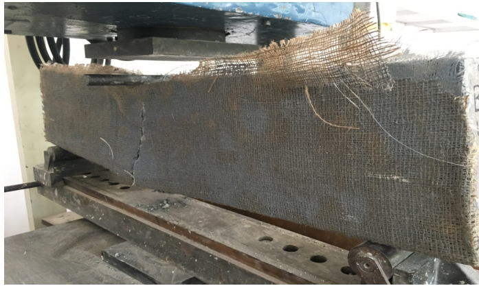
Figure 4. 14 : Showing pattern of crack at failure load of UW-B1 beam.
