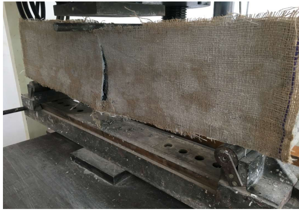
Figure 4. 10 : Showing cracks in FRP at failure load of SW-B3 beam
