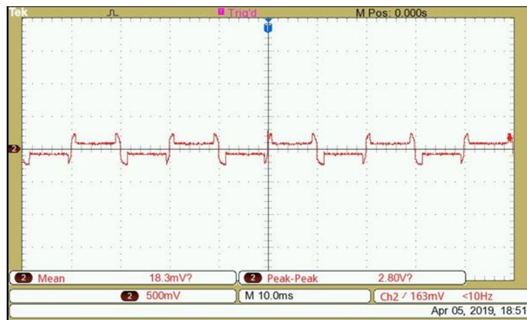
Fig. 5.9 Waveform of the triggering signal across the gate of the Triac at 40% RH.
