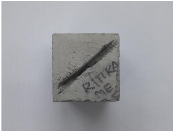
(c) Actual image of cement mortar cube with 8mm deep V-groove
