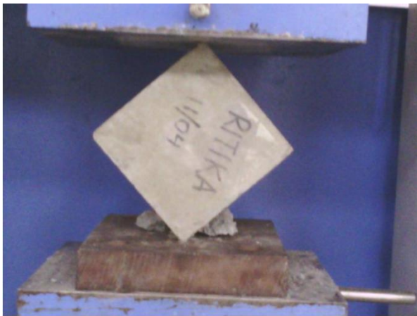
(c) Actual image at initiation of fracture
