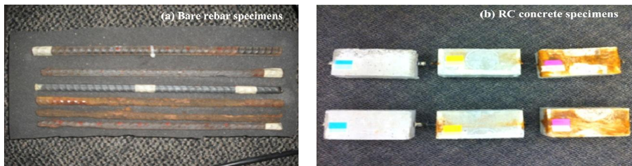
Figure 2.16: Samples of corroded specimens (a) Bare rebar specimen, (b) RC specimen [24]
