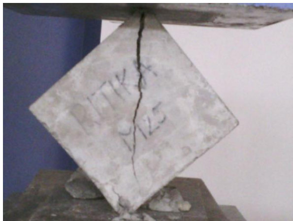
(e) Actual image after 10sec of fracture initiation
