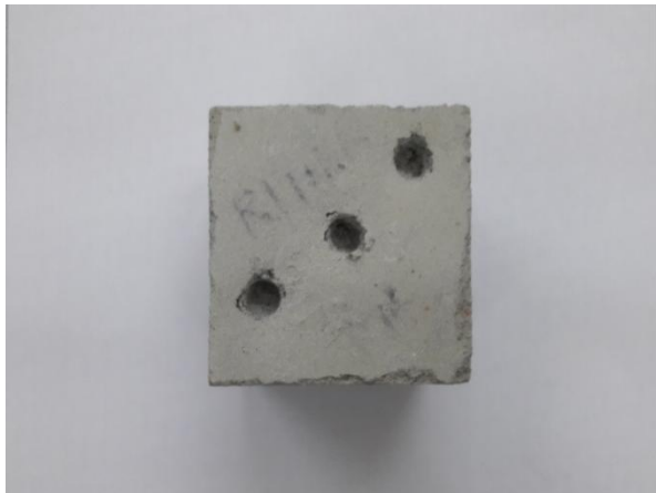
(a) Actual image of cement mortar cube with 7mm deep holes
