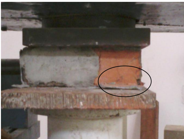
(e) Actual image at plaster detachment at the place of crack
