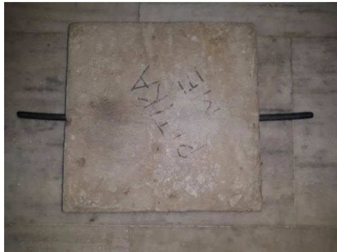
Figure 3.5: Top View of RC Slab Specimen
