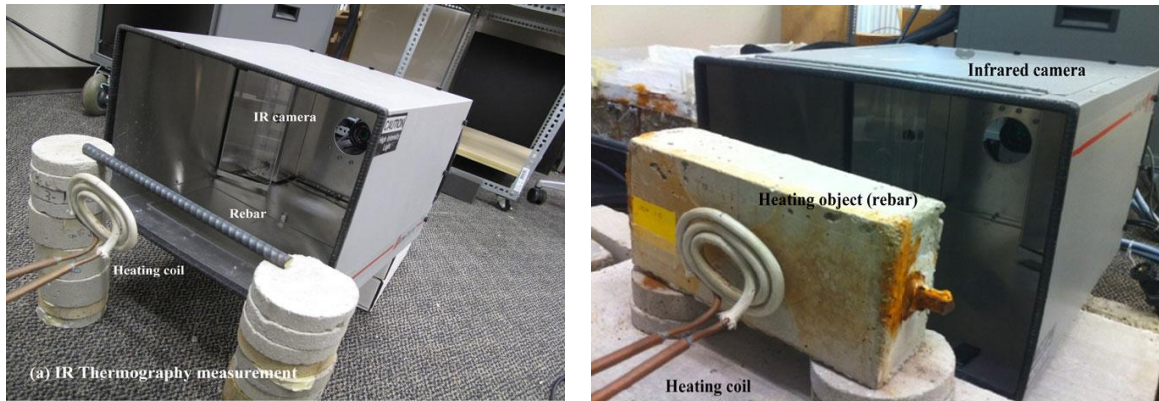
Figure 2.17: Setup for IRT for (a) Bare Bar (b) RC Specimen [24]
