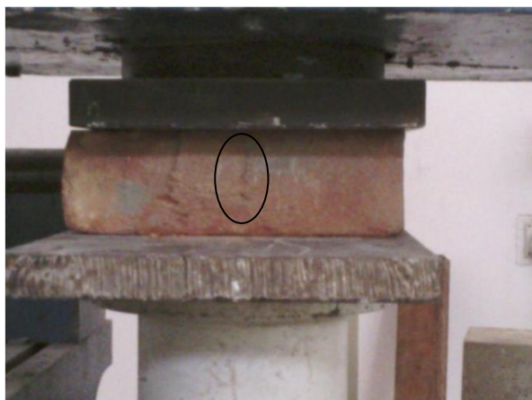
(c) Actual Image at first major crack
