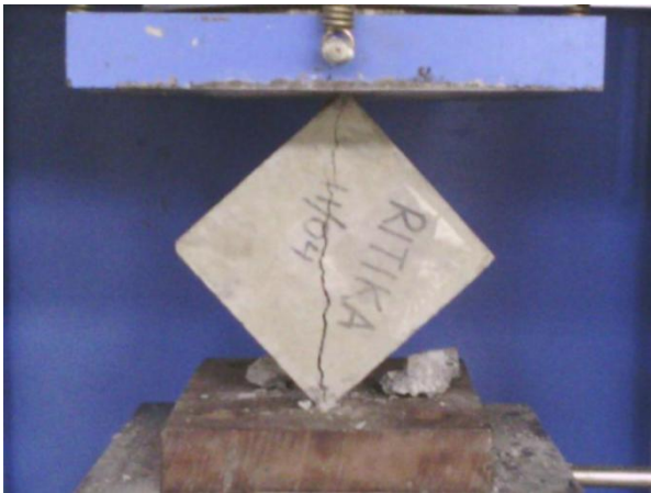
(e) Actual image after 20sec of fracture initiation
