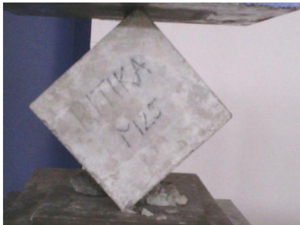
(c) Actual image at initiation of fracture
