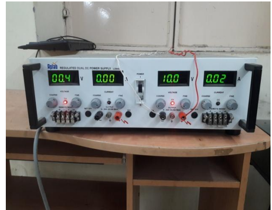
(c) Power Supply (APLAB, 64V, 0.5A)
