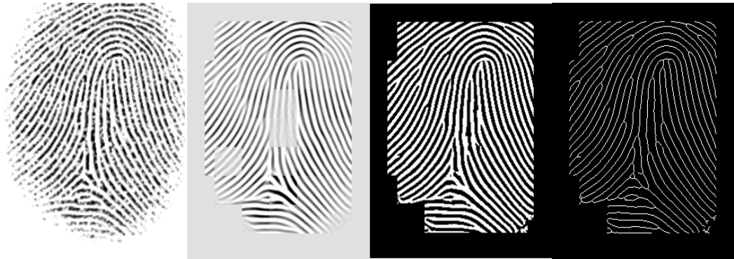
Figure 4.5: (a) Original Image, (b) Enhanced Image, (c) Binarized Image, (d) Thinned Image
