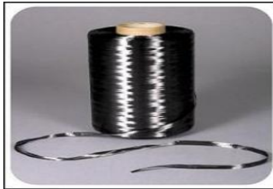
Figure 2.5: Roll of Carbon fiber [6]
