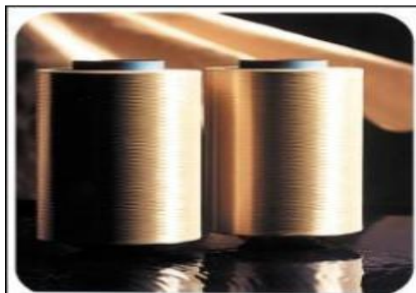
Figure 2.6: Roll of Aramid fiber [6]
