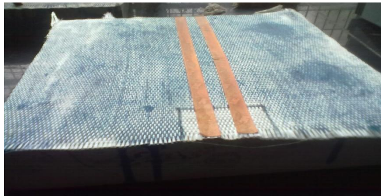
Figure 4.12 GFRP wrapped concrete with copper strips
