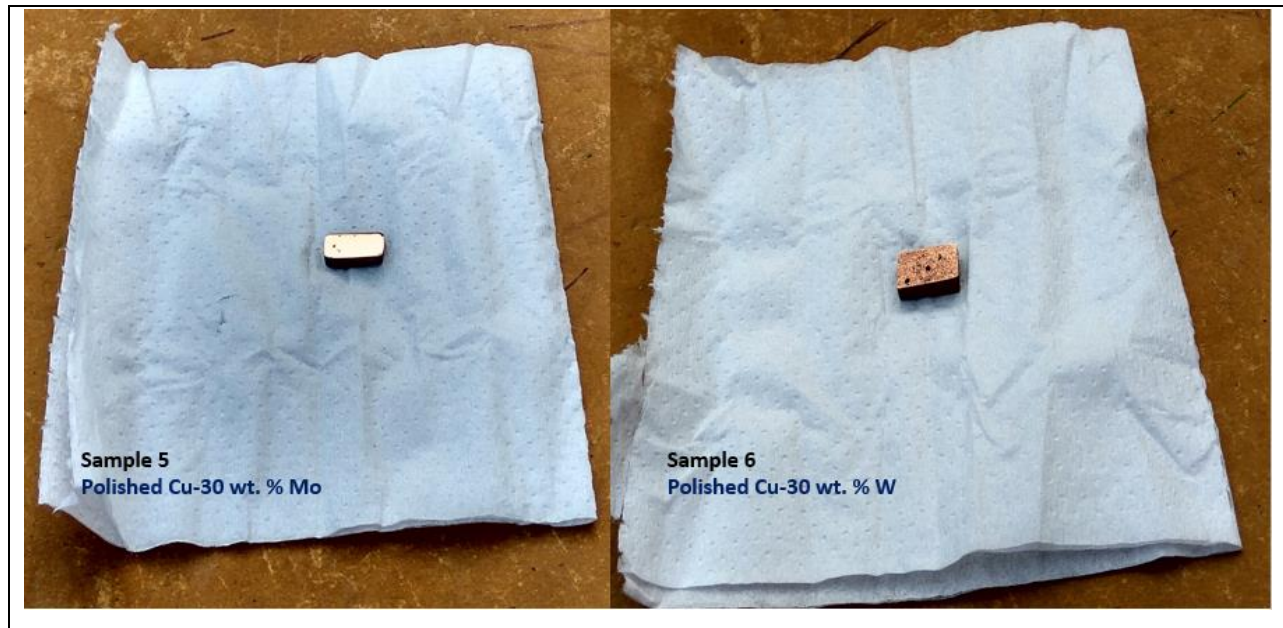
Fig. 4.17. Polished view of Cu-30 wt. % Mo and Cu-30 wt. % W samples.
