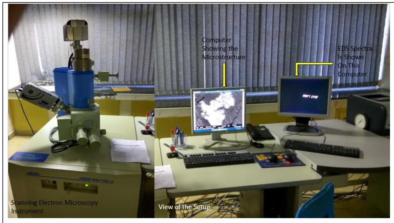
Fig. 4.19. Scanning Electron Microscope (SEM) (Courtesy: SAI Labs, Thapar University, Patiala).
