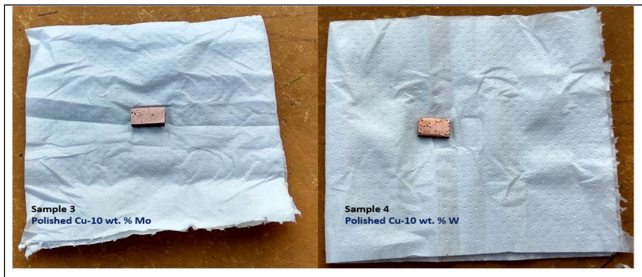
Fig. 4.16. Polished view of Cu-10 wt. % Mo and Cu-10 wt. % W samples.
