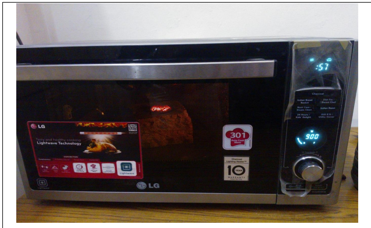
Fig. 4.10. Active microwave oven while heating the composite material at 900 W power (Courtesy: Microwave Processing Lab, Thapar University).
