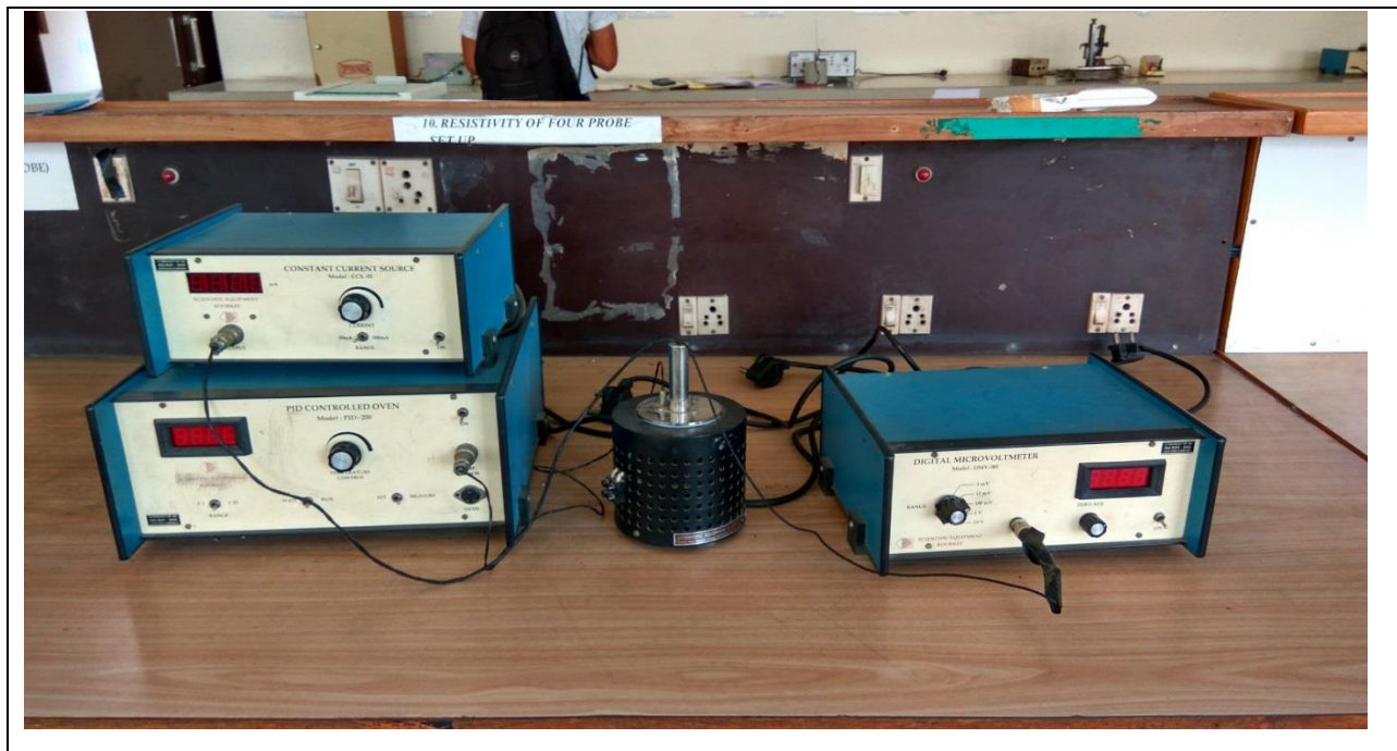
Fig. 4.26. Actual four point probe instrument (Courtesy: Material Science Lab (UG), Thapar University, Patiala).
