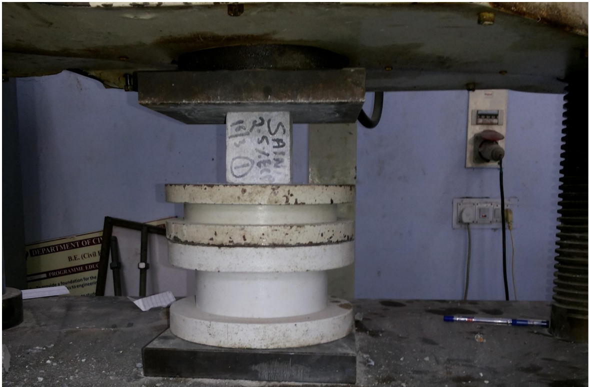
Figure 3.11: Compressive strength test in UTM
