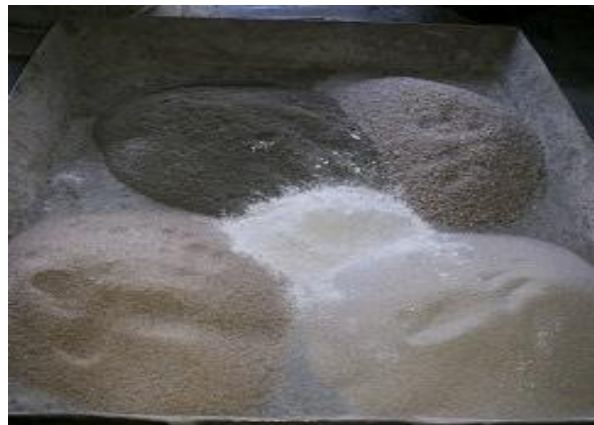
Figure 3.6: Weighted dry Cement, Sand and ESP in a dry tray
