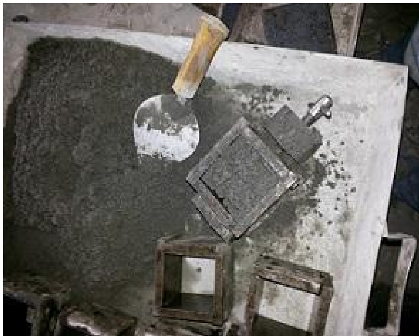
Figure 3.9: Filling of moulds with cement mortar
