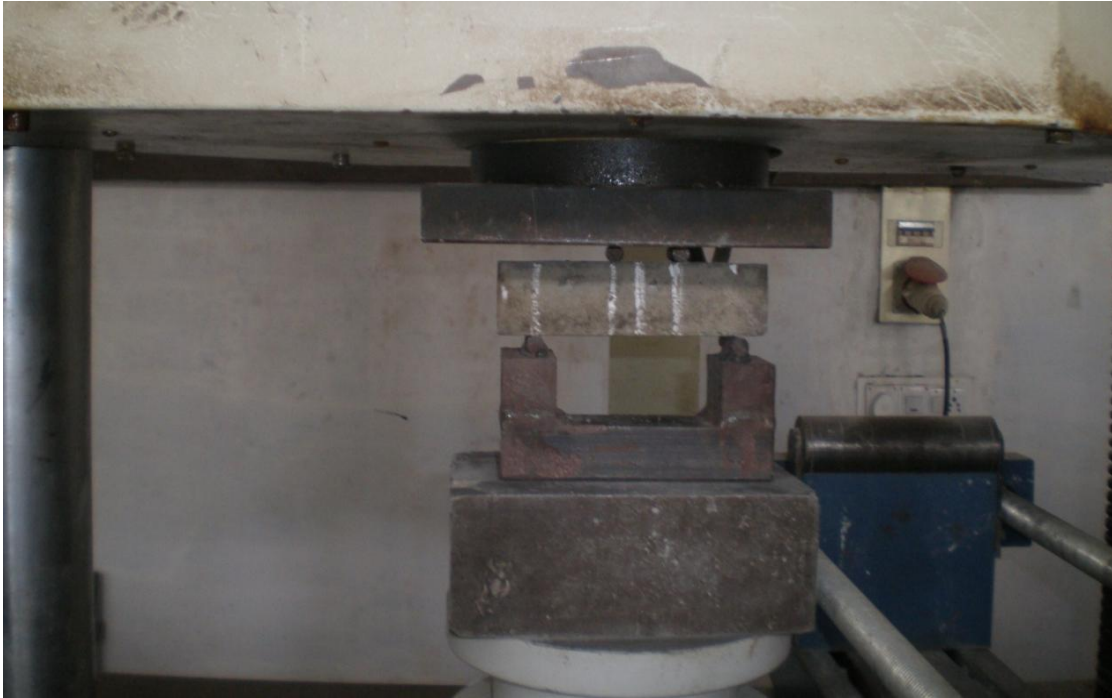
Figure 3.12: Flexural strength test on Beam in UTM
