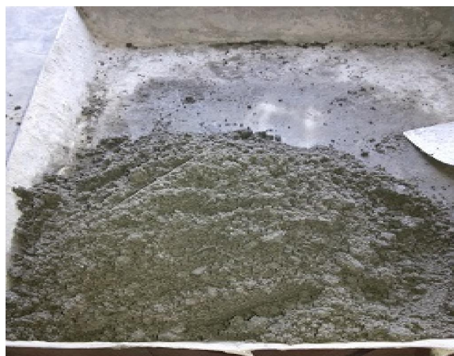
Figure 3.8: Mixing of Cement, Sand, ESP and Water in a tray.
