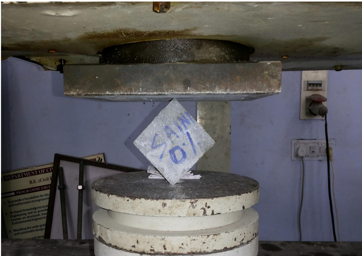
Figure 3.13: Split tensile strength test in UTM
