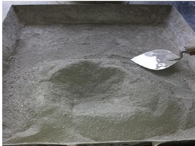
Figure 3.7: Dry mixing of Cement, Sand and ESP in a dry tray
