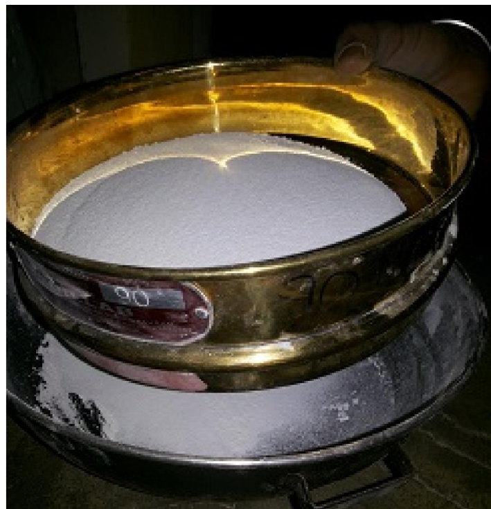
Figure 3.5: Sieving of ESP through 90 \mu\text{m} sieve obtained after grinding
