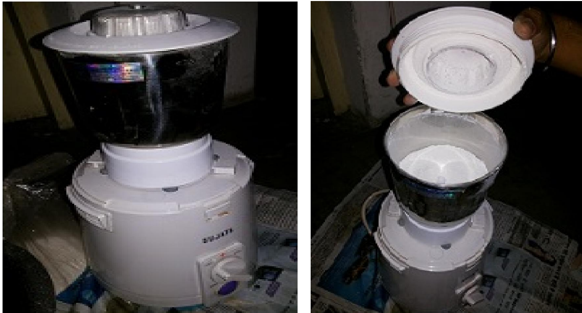
Figure 3.4: Grinding of eggshell by grinding machine
