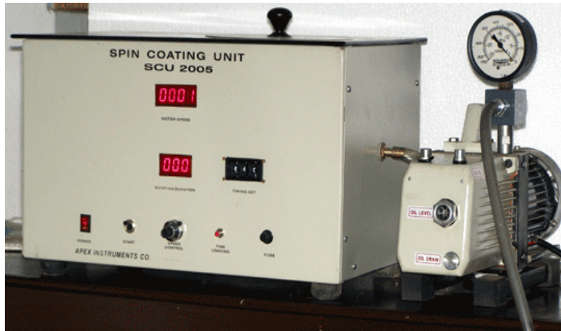
PHOTOGRAPH 3 Spin coater unit.
