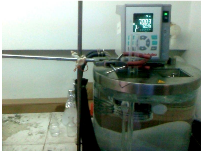
Figure No. 3.6: Ubbelohde -viscometer with temperature bath
