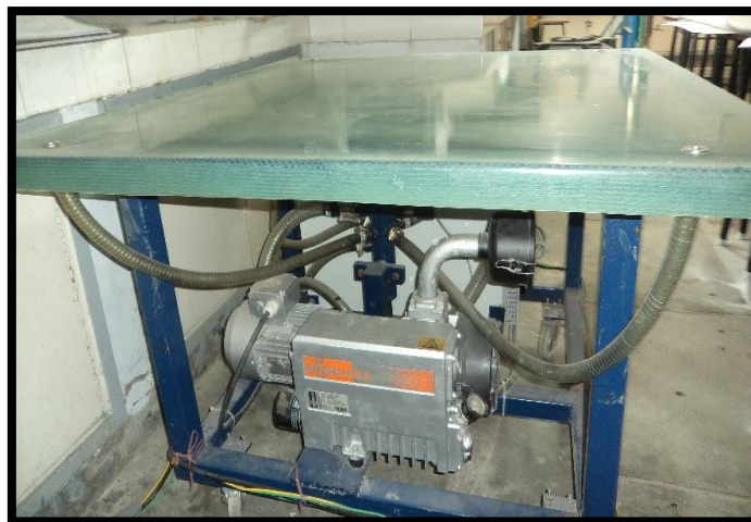
Figure 3.5: Vacuum assisted resin infusion moulding (VARIM) [Photo courtesy: Chemical Engineering Department, Thapar University, Patiala]
