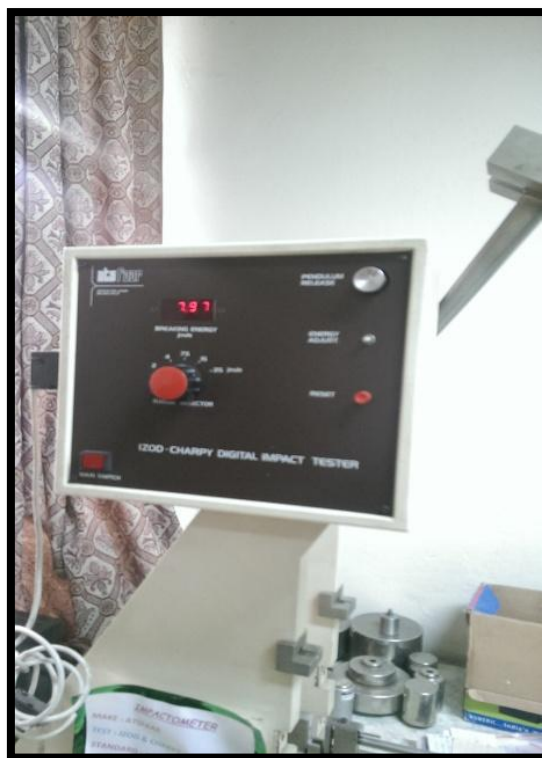
Figure 3.8: Low capacity Izod Impact Tester [Photo Courtesy: CIPET, Amritsar]
