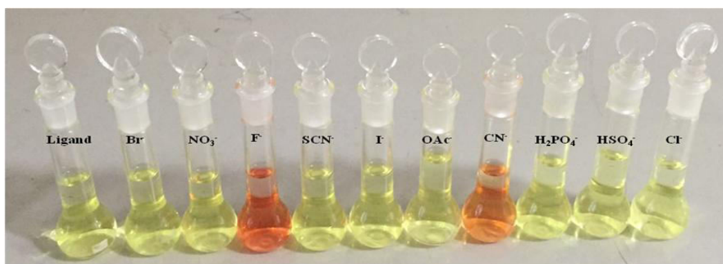
Figure 3: (b) Photographs of probe 5 in the presence of different anions at 20 \mu\text{M} in \text{CH}_3\text{CN} .
