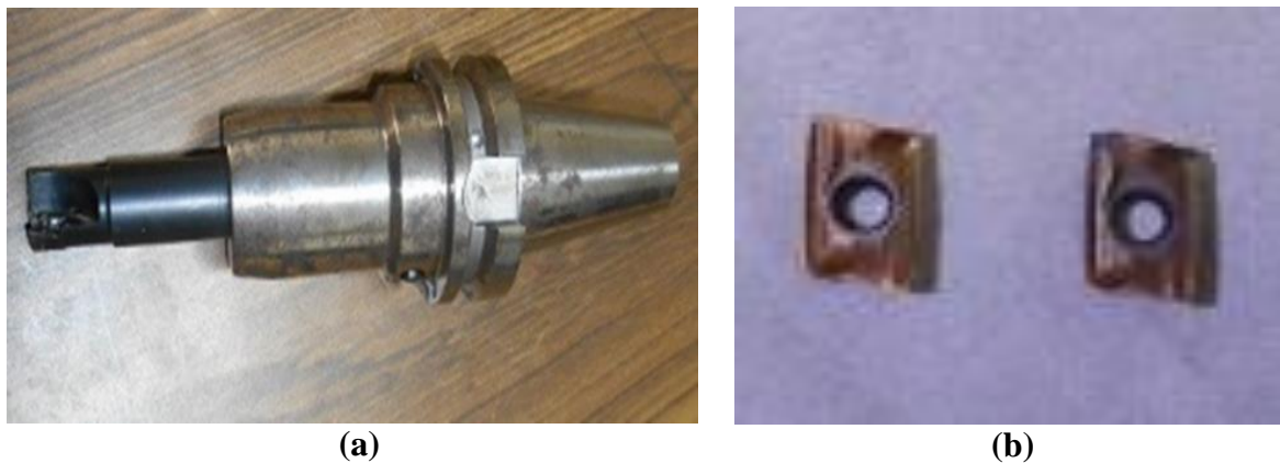
Figure 3.1: (a) CNC Tool Holder Hydro-Grip adapter T40-SHYD20-095M (b) Tungsten Carbide inserts with Titanium Aluminium Nitride (TiAlN) coating
