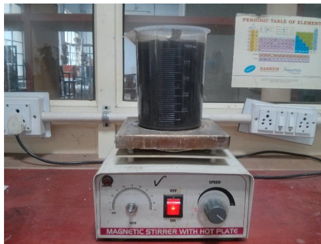
Figure 4.17: Stirring process of copper oxide (CuO) on the magnetic stirrer hot plate
