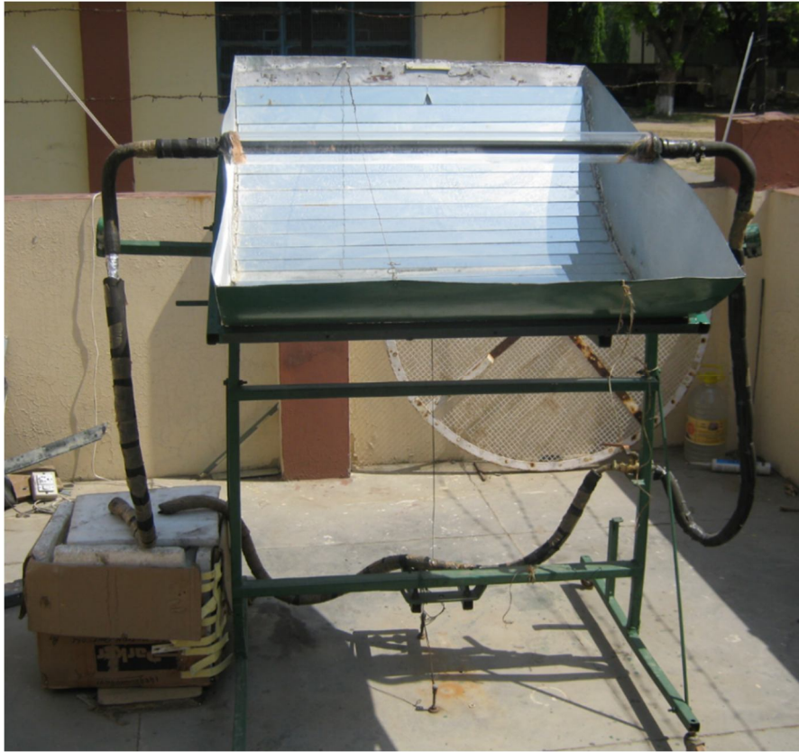
Figure 4.1: Parabolic Trough Solar Collector (PTSC) set-up
