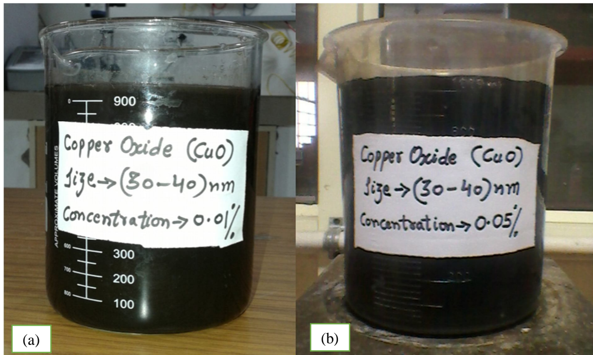
Figure 4.18 (a) & (b): Copper oxide water based (CuO) nanofluid with 0.01% & 0.05% volume concentration
