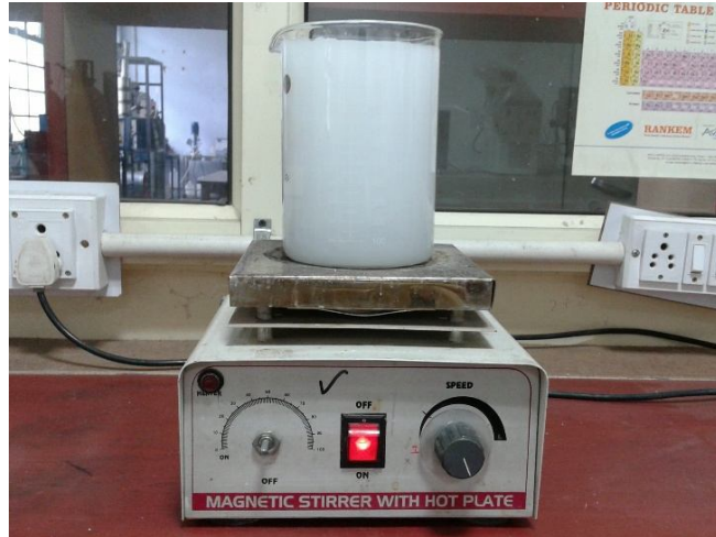
Figure 4.15: Stirring process of alumina ( \text{Al}_2\text{O}_3 ) nanofluid on Magnetic stirrer hot plate
